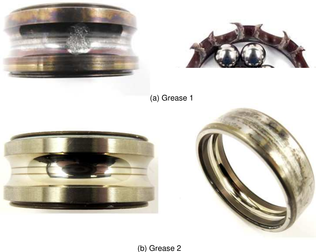
Figure 2. (a) Photographs of typical failures in the endurance tests (grease 1), indicating inner ring spalling and surface discoloration and cage (glass-fibre reinforced polyamide) overheating due to high temperatures generated on the raceways. (b) shows a non-failed bearing showing nearly zero overheating running with grease 2.
