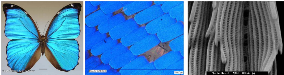
Figure 6. Example of bio-inspiration found in the world of Insects with the microscopic structure of the scales of the wings of the Morpho menelaus butterfly, which gives it an impermeability unique in the world and can be used to develop particularly hydrophobic glass surfaces (Photographs Serge Berthier).
