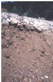
Pictures of armoring on the field resulting from size-segregation
