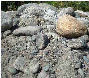
Pictures of armoring on the field resulting from size-segregation
