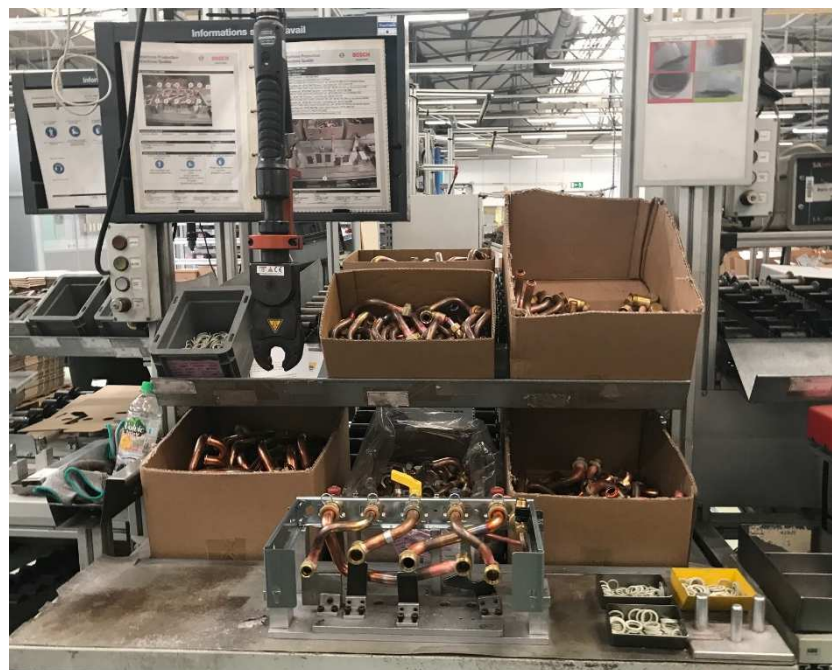
Figure 1 - A component assembly station at elm.leblanc factory, in which paper instructions (upper left part of the image) will be replaced by augmented reality instructions.
