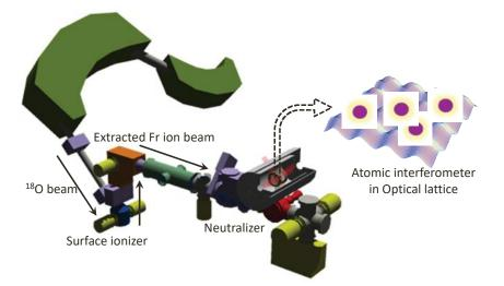
**FIGURE 1.** The overview of the EDM apparatus. The primary beam of <sup>18</sup>O is injected to the <sup>197</sup>Au target installed in the surface ionizer. The Fr produced in the target is extracted as ion, and transported to the neutralizer, and moved to the MOT and OL to measure the EDM with atomic interferometer.
