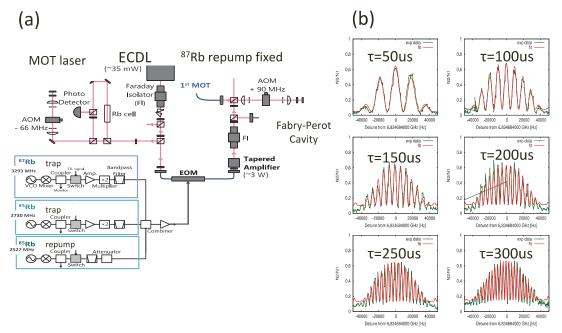
FIGURE 4. The left figure shows the laser optics for the MOT to trap the dual species atoms such as  $^{85}$ Rb and  $^{87}$ Rb with an ECDL. The right plots show the interference pattern of Ramsay resonance with the change of interaction time from 50 us to 300 us. The peak width corresponds to the resolution of the EDM measurement, and to achieve the sensitivity  $10^{-30}$ ecm, interaction time of  $1\sim10$  s will be required.
