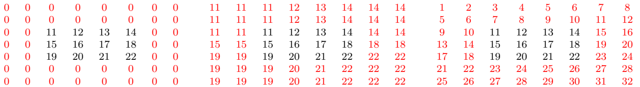
Figure 3: Illustration of the three different options for the border conditions. In grey: original image, in red: borders extension. From left to right: Dirichlet conditions, Neumann conditions, slope extension.
