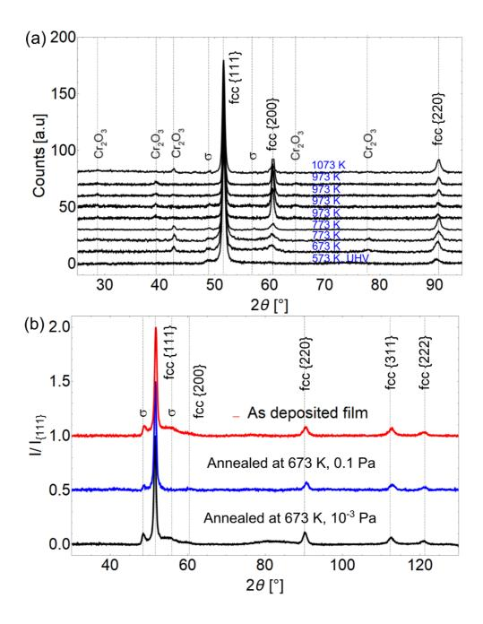
Fig. 4: Formation of  $Cr_2O_3$  leading to the disappearance of the  $\sigma$  phase (a) XRD on films annealed at different temperatures above 573 K and (b) XRD on film annealed at 673 K at different levels of vacuum.
