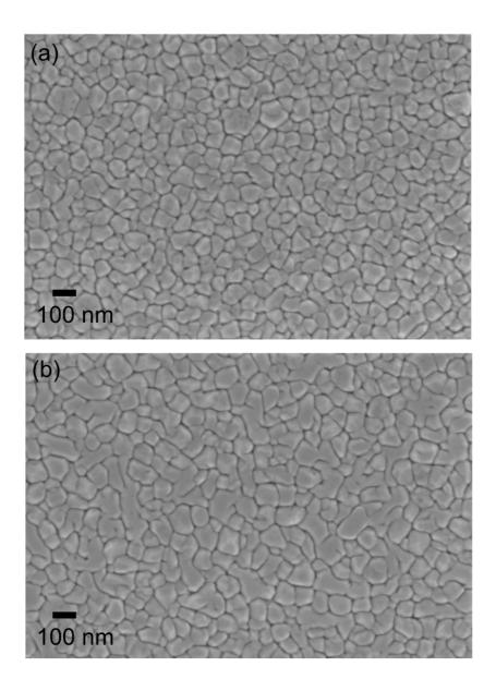
Fig 3: Typical plan view SEM images of the films deposited on (a) Si/SiO<sub>2</sub> and (b) c-sapphire at 573 K.
