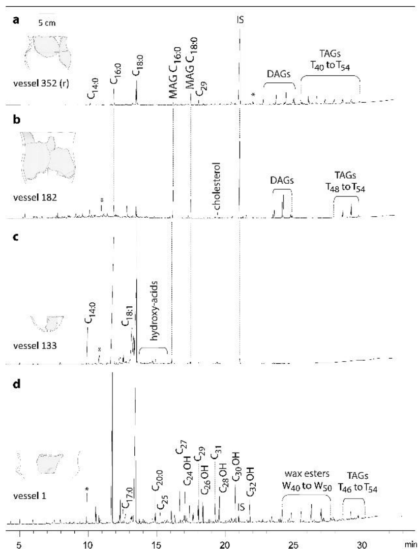
Figure 3 - Partial gas chromatograms showing typical trimethylsilylated TLEs from ves-sels from Clairvaux and containing lipid components characteristic of: (a) dairy products, (b) carcass fat, (c) plant oil, and (d) beeswax.
