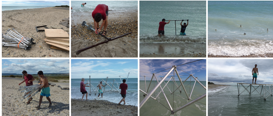
Figure 29: Deployment and in-situ tests of a prototype of one module 3 \times 3 – Villeneuve-lès-Maguelone (France).
