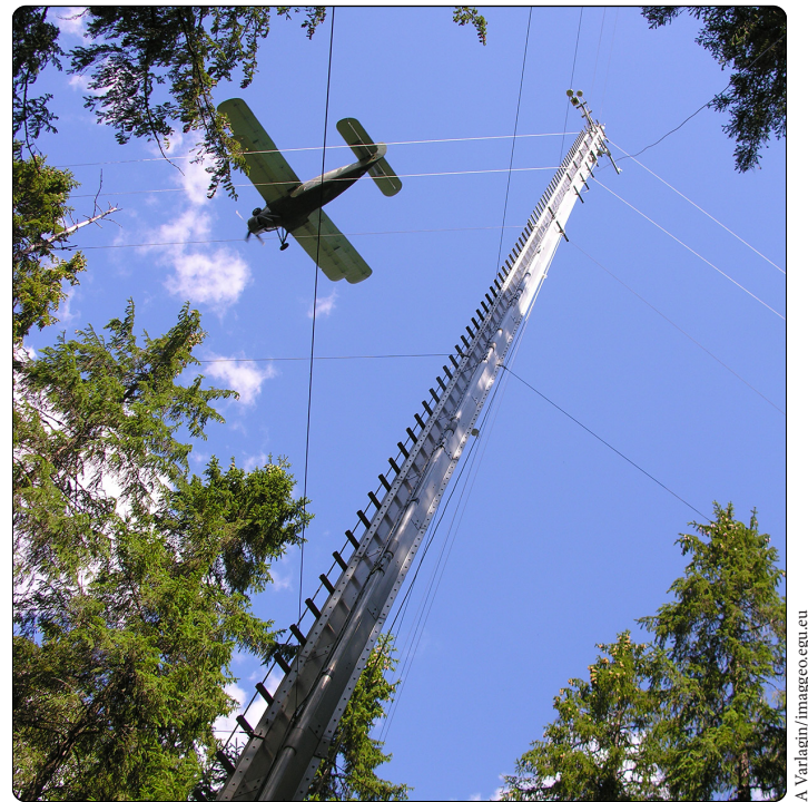
Figure 1. Image of airborne observations combined with eddy flux observations of carbon (C) fluxes to measure ecosystem–atmosphere exchanges of carbon dioxide (CO 2 ).
