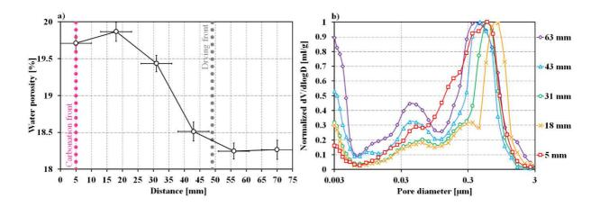
**Fig. 8.** Profiles of: (a) water porosity and (b) pore size distribution by MIP obtained after 6-month exposure.
