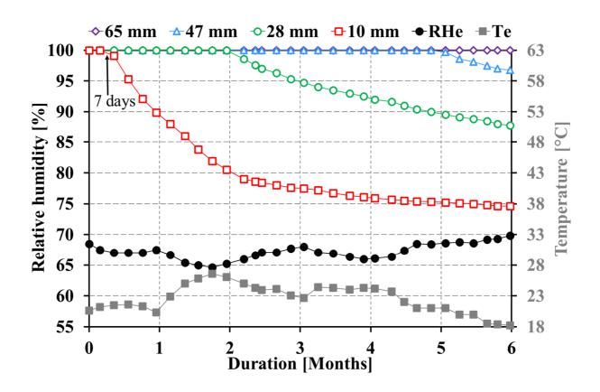
**Fig. 2.** Time-evolutions of the relative humidity at different locations inside the material, external relative humidity (RH<sub>e</sub>) and external temperature (T<sub>e</sub>) monitored during the 6-month exposure period.
