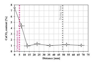
Fig. 6. Profile of CaCO<sub>3</sub> content obtained after 6-month exposure.
