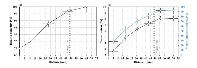
**Fig. 5.** Profiles of: (a) relative humidity, (b) water content and water saturation degree obtained after 6-month exposure.
