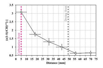
Fig. 9. Profile of carbonation potential obtained after 6-month exposure.
