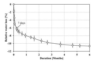
Fig. 3. Time-evolution of the relative water loss monitored during the 6-month exposure period.
