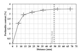
Fig. 7. Profile of Portlandite content obtained after 6-month exposure.
