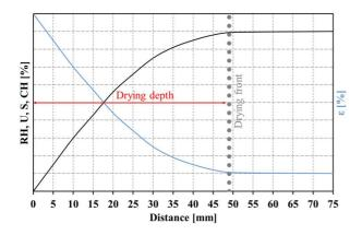
Fig. 4. Schematic presentation of the profiles of relative humidity (RH), water content (U), water saturation degree (S), Portlandite content (CH) and water porosity ( $\epsilon$ ) obtained after 6-month exposure.
