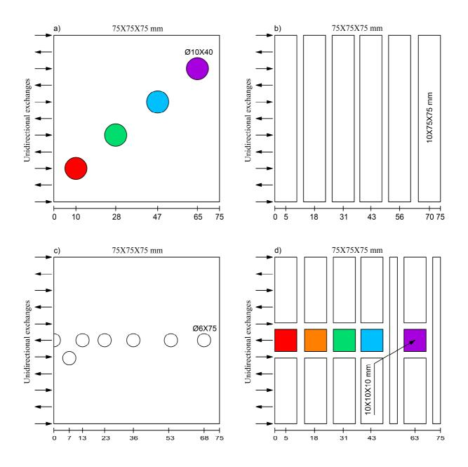
**Fig. 1.** Top views of the specimens used to determine the profiles of: (**a**) relative humidity, (**b**) water content, water saturation degree and water porosity, (**c**) CaCO<sub>3</sub> and Portlandite contents by TGA, and (**d**) pore size distribution by MIP.
