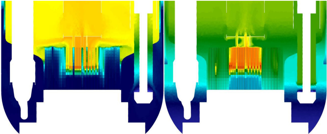
Fig. 4. Nominal and natural convection states (subchannel calculation in the core, CFD calculation in the plena and inter-wrapper region) – color is related to temperature scale as illustrative purpose; red-700K, blue-350K.
