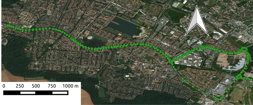
Figure 9: Generation of the test dataset in Guyancourt. Each green point indicates a location where a manually labelled LIDAR scan was recorded.
