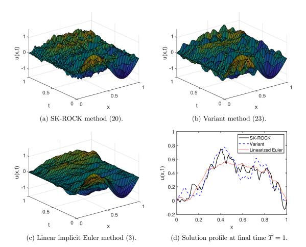
Figure 3: Samples of realisation of the stochastic nonlinear heat equation (47) with nonlinearity  $f(u) = -u - \sin(u)$  and additive noise g(u) = 1 using explicit stabilized methods (20), (23). With time and spatial stepsizes  $\tau = h = 1/100$ .
