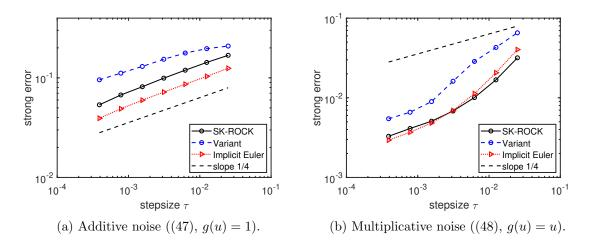
Figure 2: Strong convergence plots using SK-ROCK (20), the variant (23), and the implicit Euler method (3) for the stochastic heat equation with space-time white noise, with final time T = 0.1. Averages over  $10^4$  samples.
