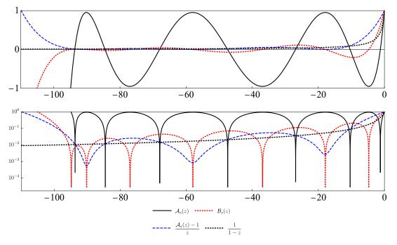
Figure 1: Stability functions  $\mathcal{A}_s(z)$  and  $\mathcal{B}_s(z)$  in (19) of the explicit stabilized methods (normal and logarithmic scales), with degree s = 7, damping parameter  $\eta = 0.05$ .
