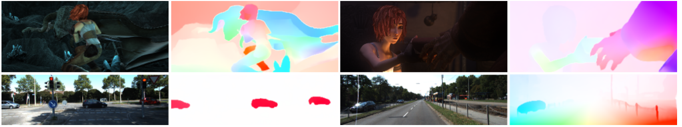
Fig. 1. Qualitative results of the proposed STaRFlow model, on MPI Sintel final pass (top line) and KITTI 2015 (bottom line) test sets. STaRFlow allows accurate motion estimation on partially occluded objects (right knee of character in upper leftmost example) and on thin objects (fingers and posts in the rightmost examples).
