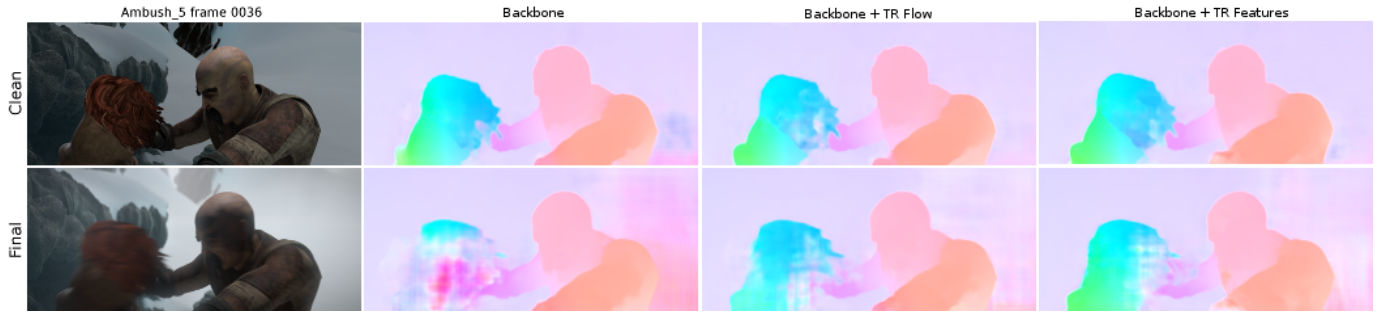
Fig. 4. Multi-frame estimation provides robustness to degraded image quality: results on Sintel clean (upper row) and Sintel Final pass (lower row).
