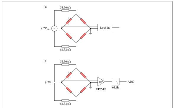
Figure 7. Electronic diagram for the cantilever measurements. The red resistor bridge is the nichrome strain bridge micro-machined on the cantilever itself. Each resistor has nearly identical impedance of order 24 k $\Omega$ . (a) Diagram for mean value measurements. The carrier wave frequency is 7 Hz, and the lock-in amplifier time constant is 1 s. (b) Diagram for fluctuation measurements. In this configuration, frequencies below  $\sim$ 10 mHz are rejected by the EPC-1B low-noise amplifier.
