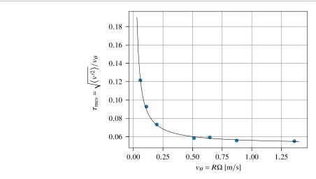
**Figure 4.** Measured turbulence intensity in He I,  $\tau_{\text{mes}}$ , computed from the hot-wire velocity signal, as a function of the azimuthal velocity. Solid line: fit using equation (7).
