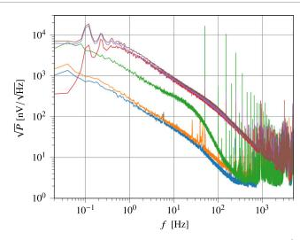
**Figure 14.** Power spectra of raw uncalibrated cantilever signal. From bottom to top:  $\Omega=0.50$  rad s<sup>-1</sup> at 1.58 K (blue), 2.0 K (orange), 2.3 K (green);  $\Omega=1.57$  rad s<sup>-1</sup> at 1.58 K (red), 1.98 K (violet), 2.3 K (maroon).
