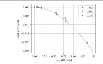
**Figure 8.** Mean cantilever signal for several mean azimuthal velocities and temperatures, both in He I (2.3 K), and in He II (1.6 K and 2.0 K). The dashed line is a quadratic fit.
