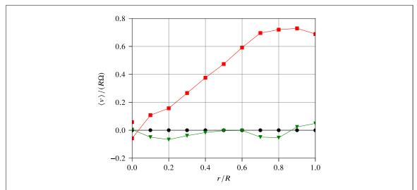
Figure 2. Velocity profiles obtained from laser Doppler velocimetry at mid-height in the SPHYNX Von Kármán cell. Red squares: azimuthal velocity; green triangles: vertical velocity; black circles: radial velocity derived from the continuity equation. The global Reynolds number is  $Re_g = 5 \times 10^5$ .
