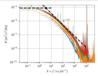
**Figure 18.** Velocity power spectra obtained in He I (2.3 K) in *co-rotation* with the hot-wire as a function of the wave number k. From bottom to top:  $\Omega = 0.19 \text{ rad s}^{-1}$ ,  $\Omega = 0.50 \text{ rad s}^{-1}$ ,  $\Omega = 2.20 \text{ rad s}^{-1}$ ,  $\Omega = 3.77 \text{ rad s}^{-1}$ . The black dot is  $k_0 = 3.48 \text{ m}^{-1}$  at the intersection of the  $k^{-5/3}$  power law and the low wave number flat spectrum.
