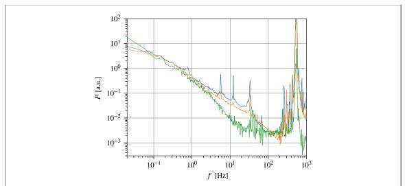
**Figure 17.** Velocity power spectra in He I and He II obtained with the miniature Pitot sensor for the angular velocity  $\Omega = 0.31 \text{ rad s}^{-1}$ . From bottom to top: 2.3 K (green), 2.0 K (orange) and 1.58 K (blue).
