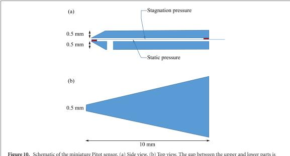
**Figure 10.** Schematic of the miniature Pitot sensor. (a) Side view. (b) Top view. The gap between the upper and lower parts is  $20 \ \mu m$ .
