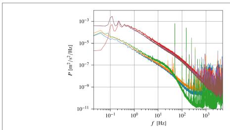
**Figure 15.** Velocity power spectra in He I and He II obtained with the cantilever with the Welch window adjusted so that 20 mHz is the lowest resolved frequency. From bottom to top:  $\Omega=0.50$  rad s $^{-1}$  at 2.3 K (green), 2.0 K (orange), 1.58 K (blue);  $\Omega=1.57$  rad s $^{-1}$  at 2.3 K (maroon), 1.98 K (violet), 1.58 K (red).
