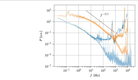
Figure 13. Power spectra obtained in He I (T = 2.30 K) at  $\Omega = 0.31$  rad s<sup>-1</sup> (bottom), and  $\Omega = 2.20$  rad s<sup>-1</sup> (top), with the hot-wire signal (light color), and the miniature Pitot signal (dark color).
