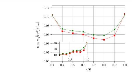
**Figure 5.** Profiles of turbulence intensity, obtained as the ratio of the standard deviation to the mean of the laser Doppler velocimetry measurements, at mid-height in the SPHYNX Von Kármán cell. Red squares: azimuthal velocity; green triangles: vertical velocity. The corresponding turbulence intensity close to the wall (r/R > 0.8) is between 5% and 10%, both for the azimuthal and the vertical components. Inset: velocity standard deviation in centimeters per second.
