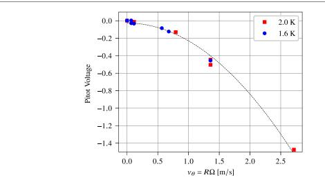
**Figure 12.** Mean voltage of the miniature Pitot sensor for several mean azimuthal velocities and temperatures in He II (1.6 K and 2.0 K). The dashed line is a quadratic fit.
