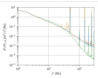
**Figure 16.** Cantilever-based velocity power spectra in He I and He II for  $\Omega = 0.50$  rad s<sup>-1</sup> with the Welch window adjusted so that 1 Hz is the lowest resolved frequency. The trend to saturation at high frequency is consistent with the expected noise floor from the electronics. Their level vary because of changes in sensor sensitivity. From bottom to top 2.3 K (green), 2.0 K (orange), 1.58 K (blue).
