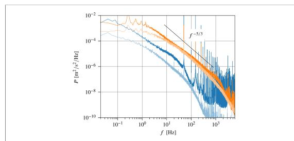
**Figure 9.** Turbulent velocity power spectra obtained with the cantilever in He I (2.3 K), using the quadratic calibration shown in figure 8 (dark lines), and the hot-wire (light lines) at angular velocities  $\Omega=0.50~{\rm rad~s^{-1}}$  (bottom) and 3.77 rad s<sup>-1</sup> (top). Black line shows the -5/3 slope.
