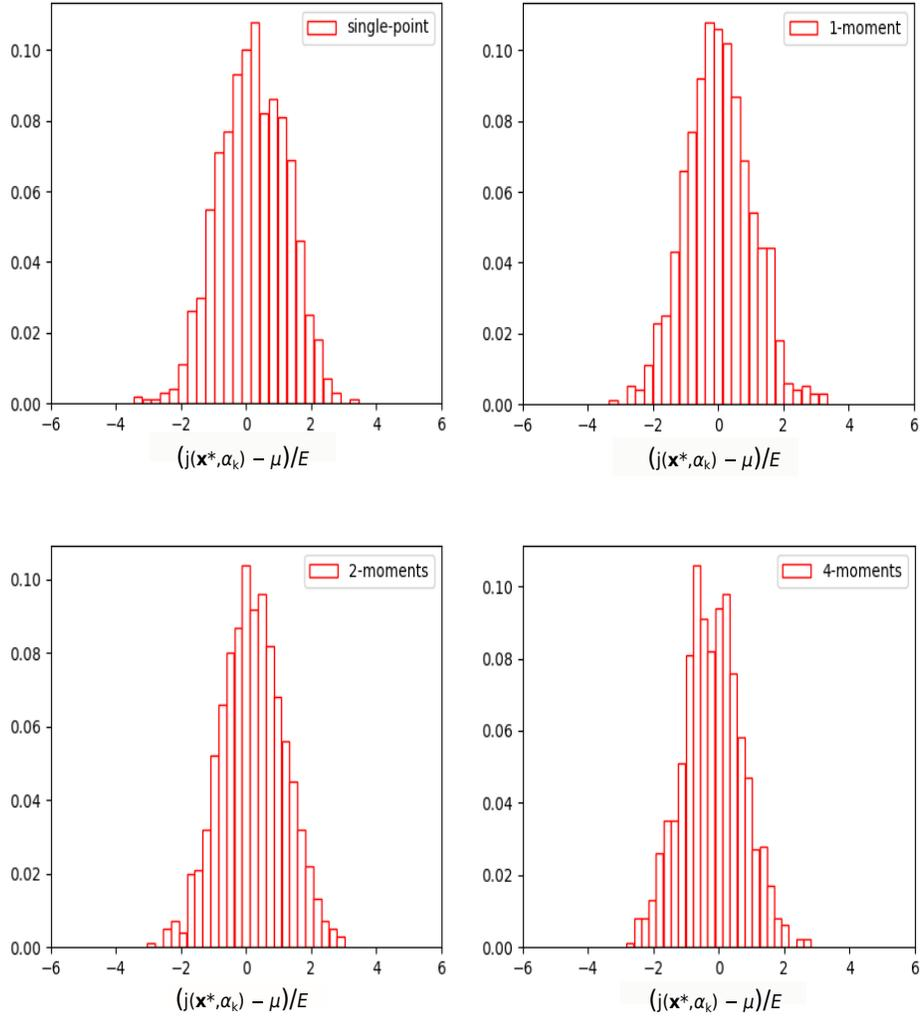
**Figure 4.** Relative frequency histogram of  $(j(\mathbf{x}^*, \alpha_{k=1, \dots, M}) - \mu) / E$  with  $M = 1000$ . Controlling all four moments reduces the variability of the functional and therefore improves the robustness of the design.
