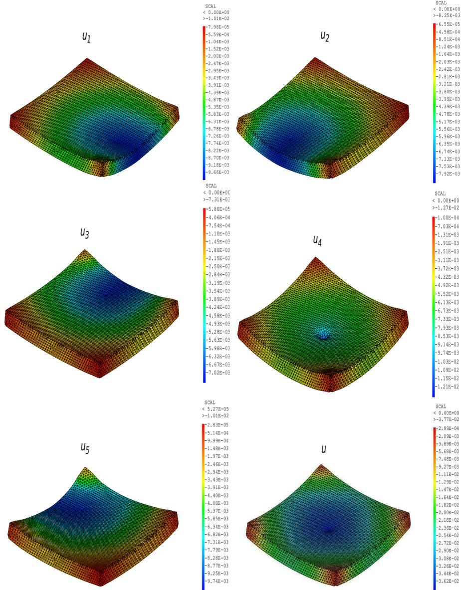
**Figure 2.** The 5 first pictures represent elementary displacements  $u_{i=1,\dots,5}$  and the bottom right picture shows the total structural displacement  $u = u_0 + \sum_{i=1}^{N=5} x_i u_i$ , where  $u_0 = 0$  in this case. The elementary displacements cannot be retrieved using symmetry considerations from each other.
