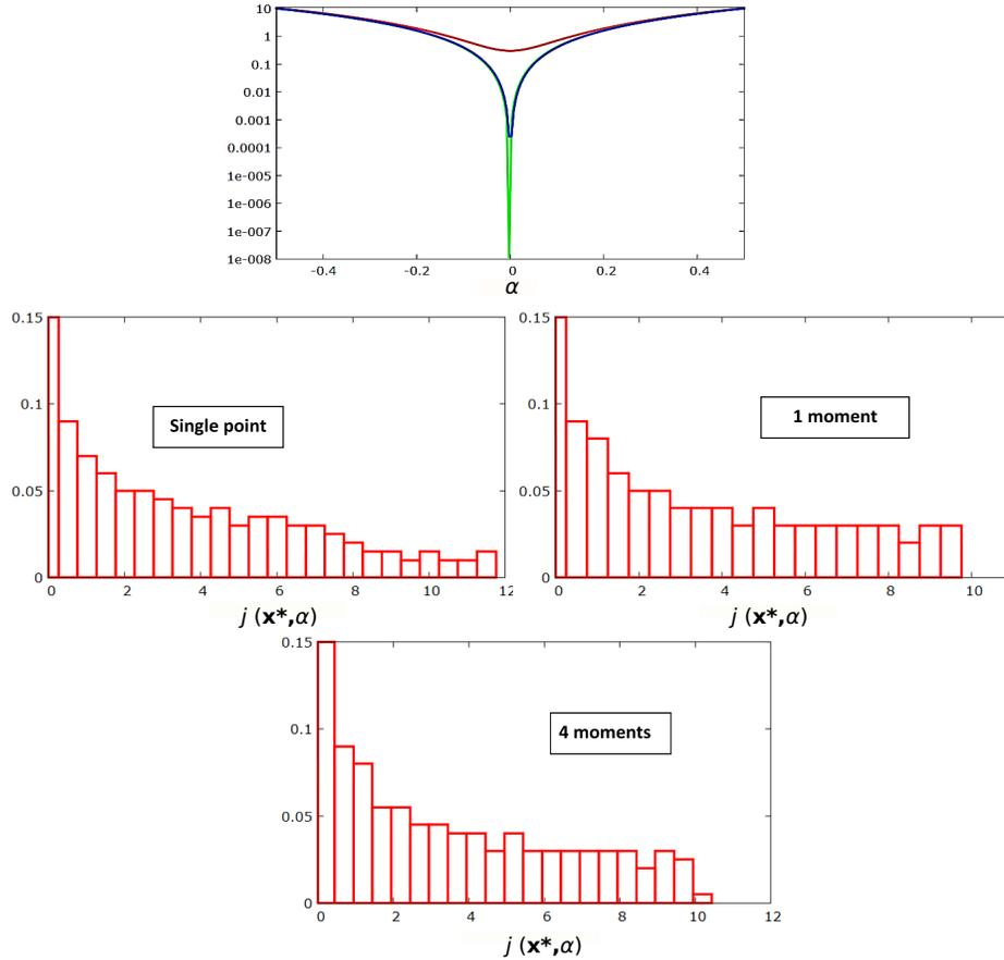
**Figure 3.** Upper: functional  $j(\mathbf{x}^*, \alpha)$  given by Equation (13) vs.  $\alpha$  for single-point optimization, mean-based and with constraints on moments two, three and four. Lower: histograms of  $j(\mathbf{x}^*, \alpha_{k=1, \dots, M})$  for a single-point minimization and when controlling one and then all first four moments.
