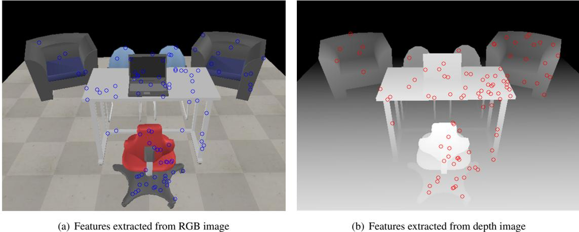
**Fig. 3.** Features extracted from RGB and depth images of camera **C1** in the multi-view system composed of 2 cameras as shown in Fig. 2. The extracted feature points are also visible to camera **C2**.
