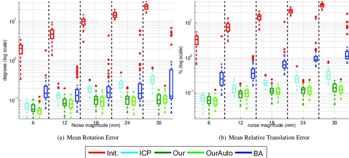
**Fig. 9.** Mean Error distribution, of pose estimates for cameras **C2**, **C3** and **C4**. in a four camera setup. 100 2D and 100 3D feature points are used. Gaussian noise is added to the data, being the variance of the 2D noise fixed ( $\sigma_{2D} = 1\text{pix}$ ), and the 3D noise  $\sigma_{3D}$  is varied between 8mm and 30mm (horizontal axes).
