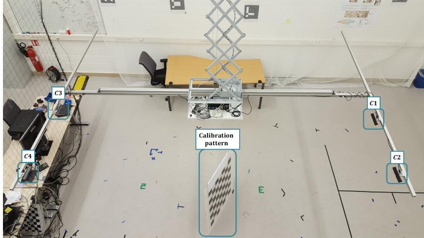
**Fig. 13.** Multi-view system consisting of 4 Asus Xtion Pro Live Cameras **C1**, **C2**, **C3** and **C4** mounted on a ceiling lift. This system is used to acquire measurements of a real scene. A two-sided planar checkerboard calibration pattern used to extract feature points is also shown.
