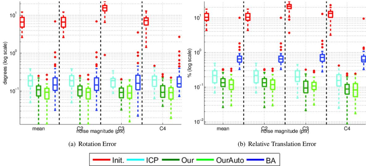
**Fig. 10.** Comparison of error distributions, of the extrinsic calibration of a four camera setup, using 100 2D and 100 3D feature points. The results are based on mean error distribution and error distribution for camera C2, camera C3 and camera C4. Gaussian noise is added to the data, being the variance of the both 2D noise and 3D noise fixed ( $\sigma_{2D} = 1\text{pix}$ ,  $\sigma_{3D} = 18\text{mm}$ ).
