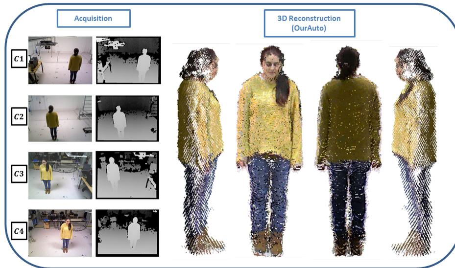
**Fig. 14.** 3D reconstruction of a human using a real scene acquired from the multi-view system shown in Fig. 13. Acquisition: Each of the 4 cameras acquire an RGB image and a depth image. 3D Reconstruction: Point clouds based 3D reconstruction using pose estimates refined by the proposed bi-objective scheme with the help of automated weighting.
