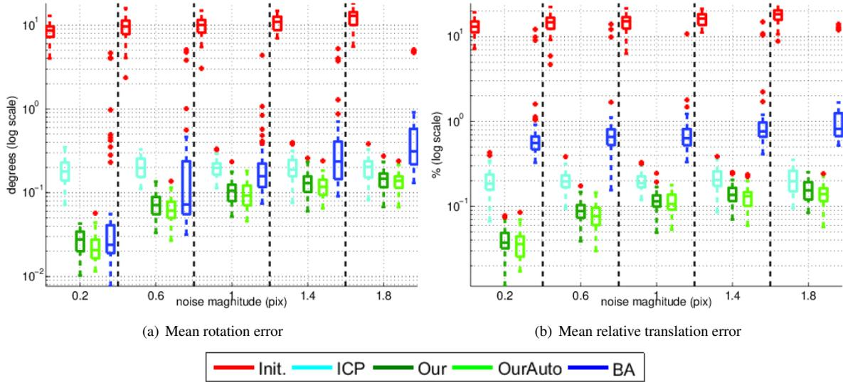
**Fig. 8.** Mean error distribution, of pose estimates for cameras **C2**, **C3** and **C4**. in a four camera setup. 100 2D and 100 3D feature points are used. Gaussian noise is added to the data, being the variance of the 3D noise fixed ( $\sigma_{3D} = 18\text{mm}$ ), and the 2D noise  $\sigma_{2D}$  is varied between 0.2 and 1.8 pixels (horizontal axes).
