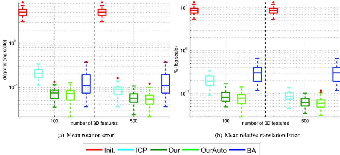
**Fig. 12.** Mean error distribution, of pose estimates for cameras **C2**, **C3** and **C4**. in a four camera setup. Gaussian noise is added to the data ( $\sigma_{2D} = 1\text{pix}$ ),  $\sigma_{3D} = 18\text{mm}$ ), 250 2D feature points and a varying number of 3D feature points (horizontal axes) is considered.
