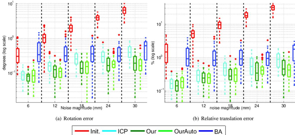
**Fig. 5.** Error distribution of pose estimates for camera **C2** in a two camera setup. 100 2D and 100 3D feature points are used. Gaussian noise is added to the data, being the variance of the 2D noise fixed ( $\sigma_{2D} = 1\text{pix}$ ), and the 3D noise  $\sigma_{3D}$  is varied between 8mm and 30mm (horizontal axes).
