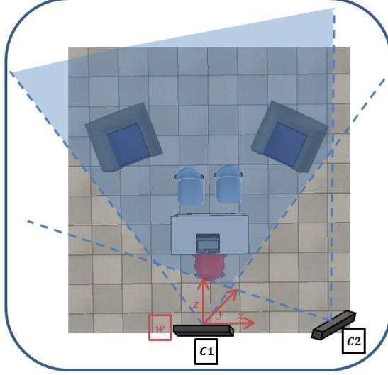
**Fig. 2.** RGB-D Multi-View System (2 cameras) with field of view (FOV) of each camera. The highlighted region represents overlapping FOVs of all cameras. The global reference frame  $w$  is aligned with camera **C1**.
