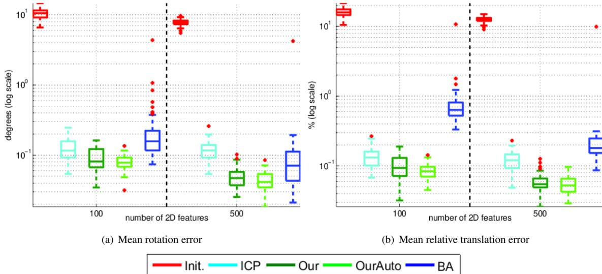
**Fig. 11.** Mean error distribution, of pose estimates for cameras C2, C3 and C4, in a four camera setup. Gaussian noise is added to the data ( $\sigma_{2D} = 1\text{pix}$ ,  $\sigma_{3D} = 18\text{mm}$ ), 250 3D feature points and a varying number of 2D feature points (horizontal axes) is considered.
