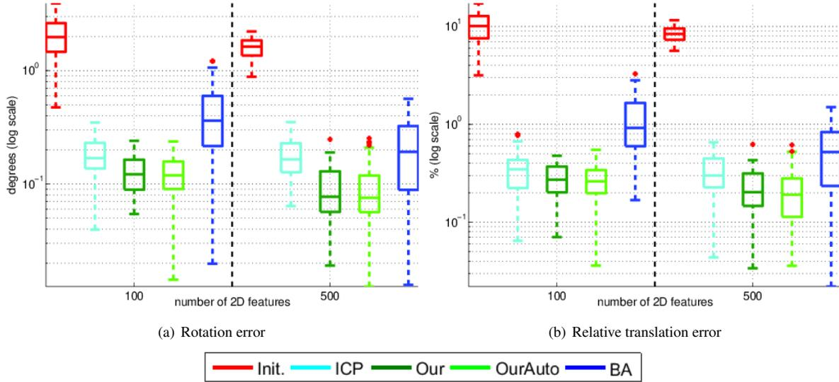
**Fig. 6.** Error distribution of pose estimates for camera *C2* in a two camera setup. Gaussian noise is added to the data ( $\sigma_{2D} = 1\text{pix}$ ,  $\sigma_{3D} = 18\text{mm}$ ), 250 3D feature points and a varying number of 2D feature points (horizontal axes) is considered.
