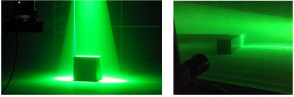
(a) The cube lighted with PIV laser sheet and LDV laser beams.
