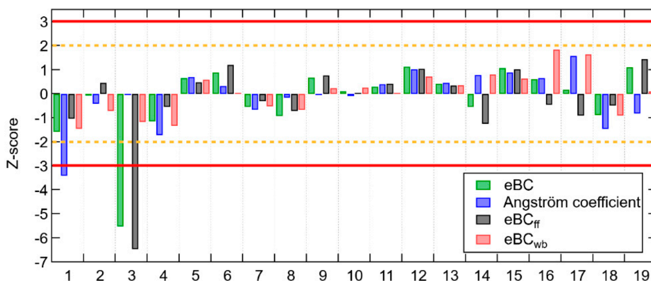
Figure 3. Z-scores obtained for BC, eBC_{ff} , eBC_{wb} concentrations and Angström exponent for 19 AE33 instruments (ordered according to increasing serial number).
