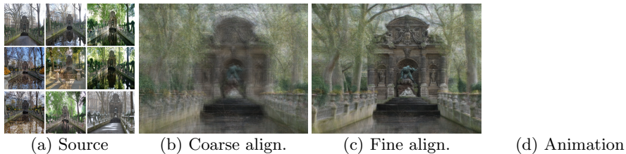
Fig. 6: Aligning a group of Internet images from the Medici Fountain, similar to [75]. We show the source images (a), the average image after coarse (b) and fine alignment (c). The animation (view with Acrobat Reader) is in (d).
