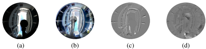
Fig. 8: Parking lot 1 of high scene DR. Desired images for pPVS: (a) LDR (b) HDR. Differences between the image at convergence and the desired image for (c) LDR- and (d) HDR-pPVS.
