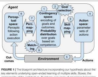
components of the architecture. Numbers: sequence of processes happening in one trial of functioning of the system.
