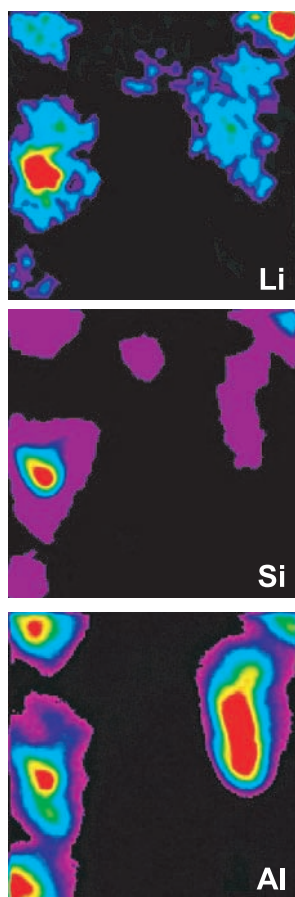
Figure 5. Example of Li-Al-Si maps performed using the 1270 ion microprobe within spots induced by previous in situ Li isotope measurements for Serie B foraminifera. In all maps, high Li signals are found to be systematically associated with high Si and Al signal. For clarity, the measured intensities have been normalized in order that the range of colors is 0–256 for all considered elements. The squares are 20 \times 20 \mu\text{m} .
