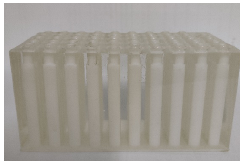
Fig.11 A resin model of the new developed pervious structure
