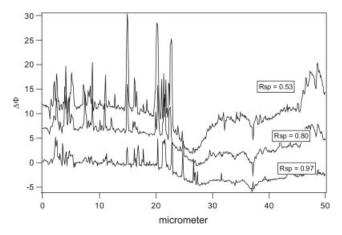
**Figure 5** Sample 2 phase profile extracted from a phase image of the interface with a partially damaged tip. The left part corresponds to BR, and the right part corresponds to SBR.  $A_0$  was equal to 178 nm. The different  $R_{sp}$  values are displayed.
