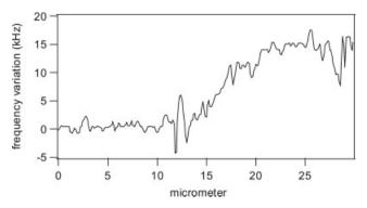
**Figure 7** Sample 2 frequency variation profile extracted from the frequency image of Figure 6. The frequency variation is displayed with a reference frequency equal to the mean frequency of the cantilever in the BR part (on the left).
