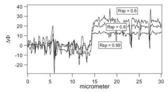
**Figure 4** Phase profile of the interface of sample 1 obtained in the tapping mode with a free amplitude equal to 180 nm, a scan frequency of 0.5 Hz, and different  $R_{sp}$  values. The left part corresponds to BR, and the right part corresponds to SBR. The phase angle deviation ( $\Delta\Phi = \Phi - \Phi_0$ ) is displayed with  $\Phi_0$  equal to the mean phase of the BR part.
