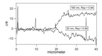
**Figure 3** Two-phase profiles extracted from the two-phase images of the interface of sample 2. The left part corresponds to BR, and the right part corresponds to SBR.  $A_0$  and  $R_{sp}$  are displayed. The phase angle deviation ( $\Delta\Phi = \Phi - \Phi_0$ ) is displayed with  $\Phi_0$  equal to the mean phase of the BR part.
