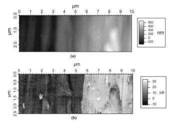
Figure 2 (a) Topography and (b) phase images of sample 1 acquired with a free amplitude of 175 nm, an  $R_{sp}$  value of 0.85, and a sweeping frequency of 1 Hz. The left part corresponds to BR, and the right part corresponds to SBR. The Z-axis scale is displayed with the corresponding color for the topography image and phase image. The phase angle deviation ( $\Delta\Phi=\Phi-\Phi_0$ ) is displayed in degrees with  $\Phi_0$  equal to the mean phase of the BR part.
