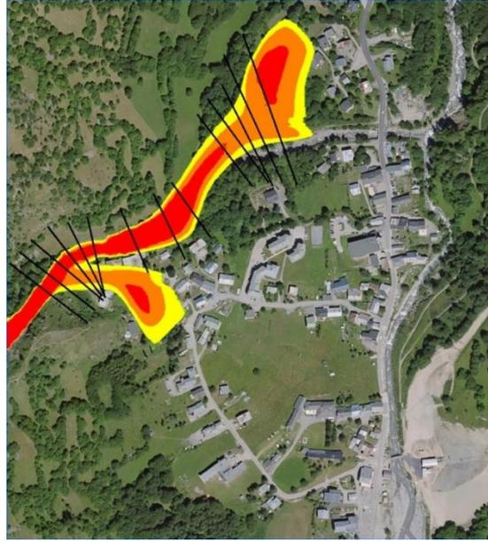
Fig. 7. Tentative example of computation of the area affected by debris flows for a single scenario, this example of a 50,000 m<sup>3</sup> debris-flow spreading computed using a rough DEM is given for illustrative purpose only.
