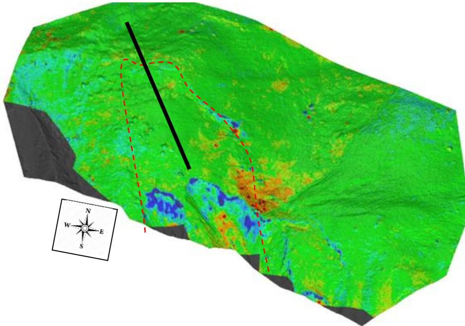
Fig. 2. Difference between the November 2015 and July 2018 photogrammetric surveys. Red: accumulation. Blue: erosion. The maximum motion is 1.5 m and the displaced volume is estimated at 230 m<sup>3</sup>. The red dashed line gives an approximate delineation of the landslide. The black line marks the position of the seismic tomography profile (see section 3.2.)
