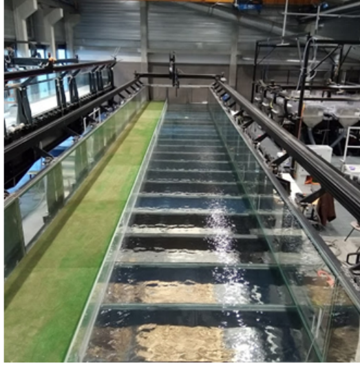
Figure 1. Open-channel flume located in the Hydraulics and Hydro-morphology Laboratory (HHLab) at INRAE, Lyon-Villeurbanne. Experiments with a working length = 18 m and a working width = 2 m (right-hand 2/3 of the total flume width with bed and sidewalls made of glass).
