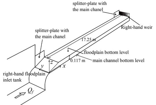
FIGURE 2. (Colour online) Inflow conditions: (a) inlet tanks; (b) sketch of the right-hand floodplain viewed from upstream. The inflow discharge in the main channel is denoted  $Q_m$ , and  $Q_f$  is the discharge in each of the two floodplains.
