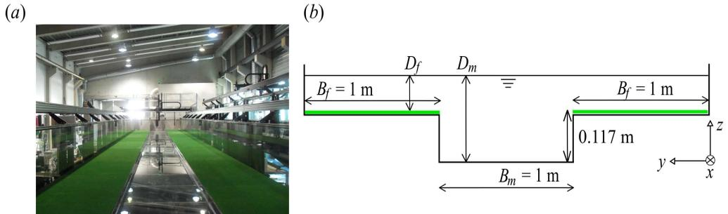
FIGURE 1. (Colour online) Compound open-channel flume (18 m  $\times$  3 m) at Irstea Lyon-Villeurbanne, France: (a) view upstream; and (b) sketch of a cross-section (view downstream), in which  $D_m$  and  $D_f$  are the flow depths in the main channel and floodplain, respectively. Shaded areas (shown in green in online version) represent artificial grass on floodplains.
