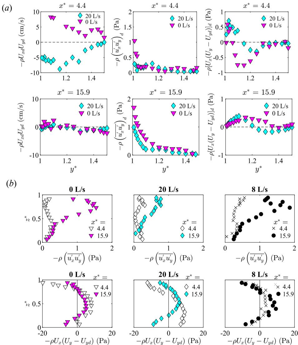
FIGURE 19. (a) Transverse distributions of depth-averaged momentum fluxes by the transverse currents,  $-\rho U_{xd}U_{yd}$ , by the shear layer turbulence,  $-\rho(\overline{u'_x u'_y})_d$ , and by the SCs,  $-\rho[U_x(U_y - U_{yd})]_d$ , for 20 L/s ( $\diamond$ ) and 0 L/s ( $\nabla$ ). (b) Vertical distributions of  $-\rho\overline{u'_x u'_y}$  and  $-\rho U_x(U_y - U_{yd})$  at  $y^* = 1.06$  for 0, 20, and 8 L/s.
