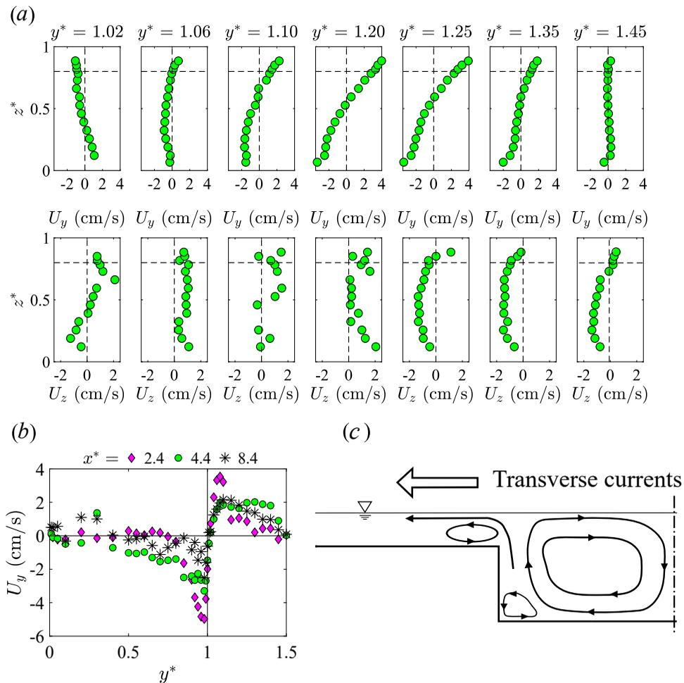
FIGURE 11. (Colour online) Case 4 L/s: (a) vertical distributions of the time-averaged transverse velocity,  $U_y$ , and vertical velocity,  $U_z$ , at  $x^* = 4.4$ ; (b) transverse distributions of  $U_y$  at elevation  $z^* = 0.91$  and at various  $x^*$ -positions; and (c) sketch of the SCs patterns in the half-MC at  $x^* = 4.4$  (upstream view). The standard errors in  $U_y$  and  $U_z$  are around 9% and 16%, respectively.
