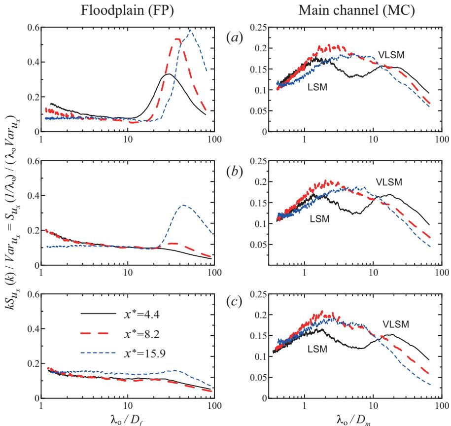
FIGURE 17. One-dimensional pre-multiplied spectra of streamwise velocity fluctuations for flow cases: 4 L/s (a); 8 L/s (b); and 16 L/s (c).  $\lambda_0$  is wavelength of a spectral component;  $Var u_x$  is variance of the streamwise velocity.
