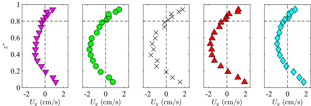
FIGURE 22. Vertical distributions of the time-averaged transverse velocity,  $U_y$ , at  $y^* = 1.06$  (in MC) and  $x^* = 15.9$ , for cases: 0 L/s (▽); 4 L/s (o); 8 L/s (x); 16 L/s (△); and 20 L/s (◇). The standard sampling error in  $U_y$  is around 9%.
