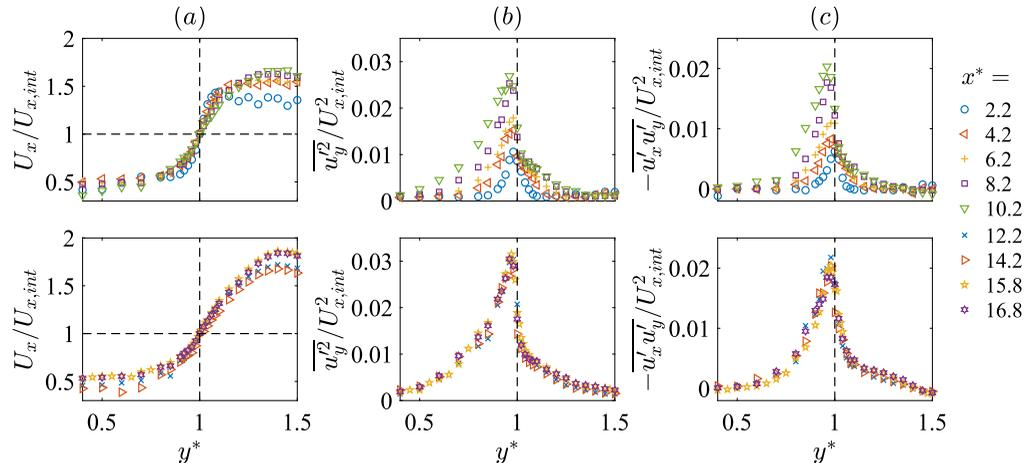
FIGURE 6. (Colour online) Transverse distributions of dimensionless (a) mean streamwise velocity,  $U_x/U_{x,int}$ , (b) transverse squared turbulence intensity,  $\overline{u_y'^2}/U_{x,int}^2$ , and (c) transverse Reynolds shear stress,  $-\overline{u_x' u_y'}/U_{x,int}^2$ , all at elevation  $z^* = 0.94$  for the case of  $8 \text{ L s}^{-1}$ . The standard errors in  $U_x$ ,  $\overline{u_y'^2}$ , and  $-\overline{u_x' u_y'}$  are around 1%, 4%, and 10%, respectively.
