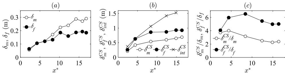
FIGURE 13. Case 8 L/s, elevation  $z^* = 0.94$ : (a) shear layer widths based on mean velocity distribution in the MC,  $\delta_m$ , and over the FP,  $\delta_f$ ; (b) characteristic scales of KHCSs in the MC,  $\delta_m^{CS}$ , in the FP,  $\delta_f^{CS}$ , and along the interface,  $\delta_{int}^{CS}$ ; (c) ratios  $\delta_m^{CS}/\delta_m$  and  $\delta_f^{CS}/\delta_f$ .
