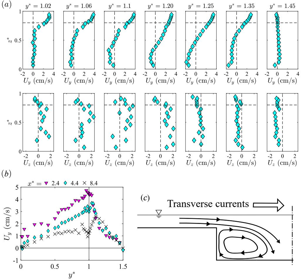
FIGURE 10. Case 20 L/s: (a) vertical distributions of the time-averaged transverse velocity,  $U_y$ , and vertical velocity,  $U_z$ , across a half-MC at  $x^* = 4.4$ ; (b) transverse distribution of  $U_y$  at  $z^* = 0.91$  and  $x^* = 2.4, 4.4,$  and  $8.4$ ; (c) sketch of the SC pattern in the half-MC at  $x^* = 4.4$  (upstream view). The standard errors in  $U_y$  and  $U_z$  are around 9% and 16%, respectively.
