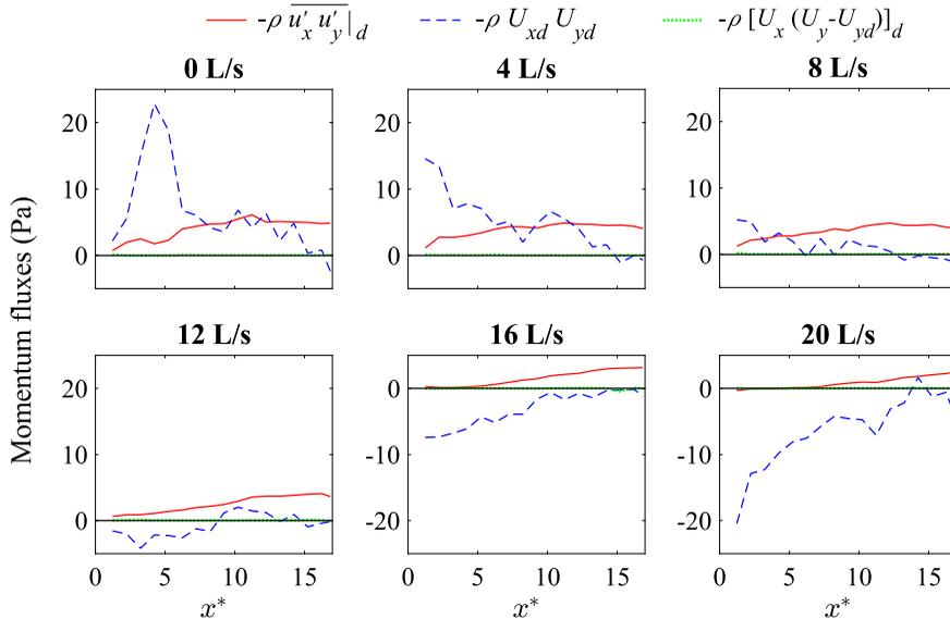
FIGURE 18. Contributions of shear layer (planform) turbulence ( $-\rho \overline{u'_x u'_y}|_d$ ), transverse currents ( $-\rho U_{xd} U_{yd}$ ) and secondary currents ( $-\rho [U_x (U_y - U_{yd})]_d$ ) to the total depth-averaged momentum exchange  $\tau_{tot}$  (i.e., terms of Eq. 7.1). Measurements are taken at the interface.
