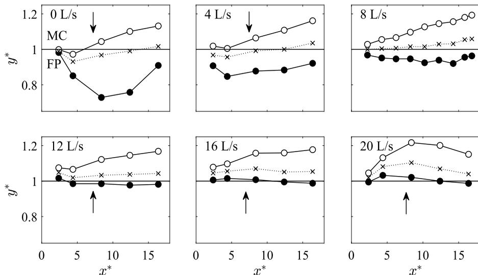
FIGURE 8. Half shear layer width,  $\delta_0/2$  (normalized by  $B_f$ ), bounded by the transverse positions:  $y_{25\%}$  ( $\bullet$ ); and  $y_{75\%}$  ( $\circ$ ). Position  $y_{50\%}$  ( $\times$ ) is also plotted. Measurements are at  $z^* = 0.94$  for the case of 8 L/s, and at  $z^* = 0.91$  for the other cases. Arrows indicate the direction of transverse currents.
