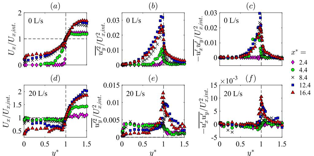
FIGURE 7. Transverse profiles of dimensionless time-averaged streamwise velocity,  $U_x/U_{x,int}$ , transverse squared turbulence intensity,  $\overline{u_y^2}/U_{x,int}^2$  and transverse Reynolds shear stress,  $-\overline{u_x u_y}/U_{x,int}$ , at various  $x^*$ -positions and at  $z^* = 0.91$  for the cases of (a-c) 0 L/s, and (d-f) 20 L/s. The standard errors in  $U_x$ ,  $\overline{u_y^2}$ , and  $-\overline{u_x u_y}$  are around 1%, 4%, and 10%, respectively.
