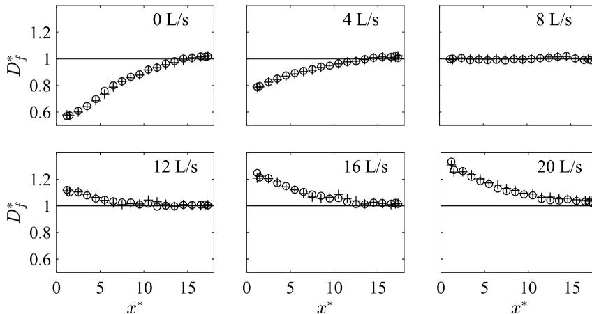
FIGURE 4. Dimensionless flow depth,  $D_f^*$ , against streamwise coordinate,  $x^*$ , at:  $y^* = 0.3$  ( $\circ$ ); and  $y^* = 0.7$  ( $+$ ). The maximum uncertainty in  $D_f^*$  is approximately  $8 \times 10^{-3}$ .
