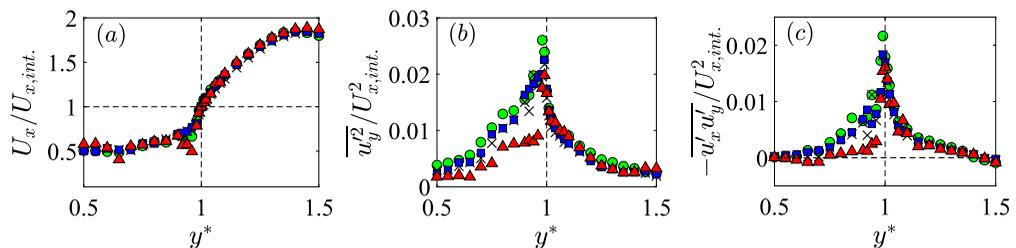
FIGURE 21. Transverse profiles of dimensionless (a) mean streamwise velocity,  $U_x/U_{x,int.}$ , (b) transverse turbulence intensity,  $\overline{u_y^2}/U_{x,int.}^2$ , and (c) transverse Reynolds shear stress,  $-\overline{u_x u_y'}/U_{x,int.}^2$ , at  $x^* = 16.4$  and  $z^* = 0.91$  for cases 4 L/s (o), 8 L/s (x), 12 L/s (□), and 16 L/s (△). The standard errors in  $U_x$ ,  $\overline{u_y^2}$ , and  $-\overline{u_x u_y'}$ , are around 1%, 4%, and 10%.
