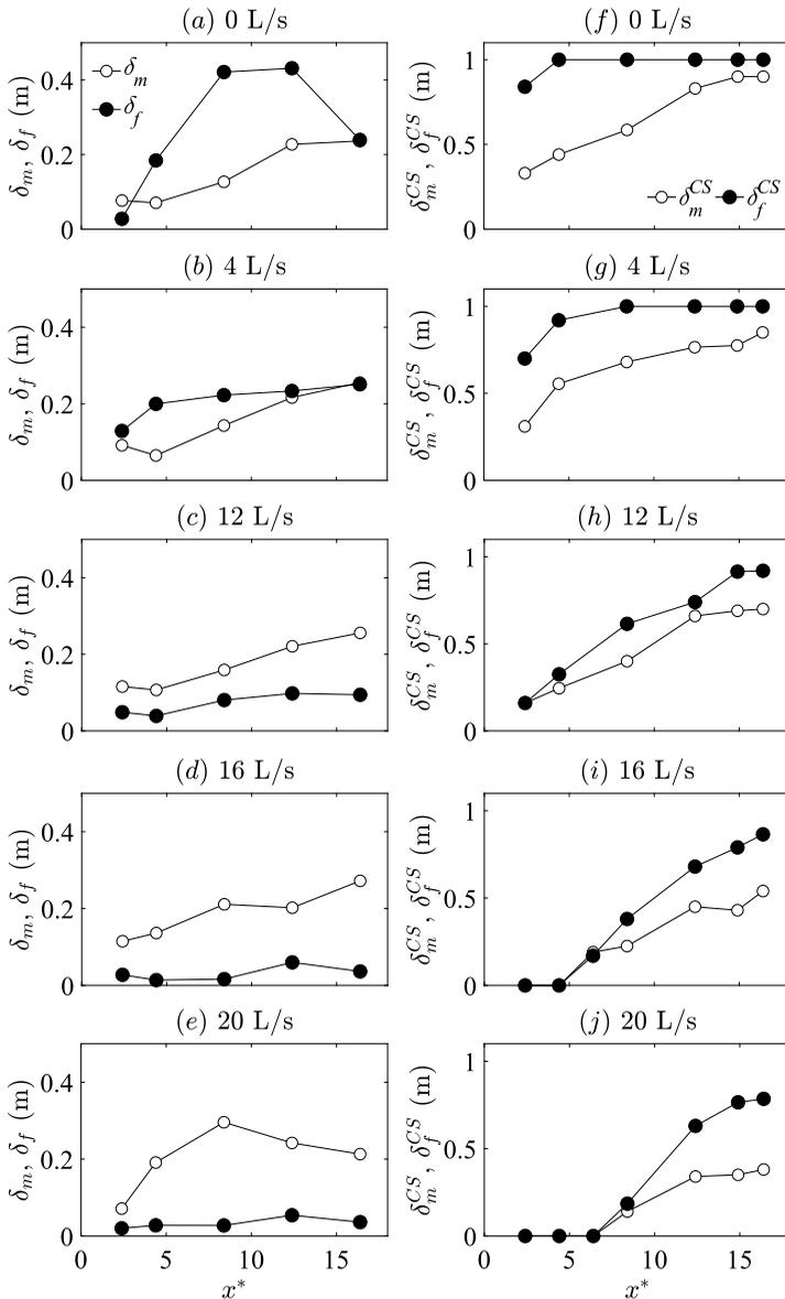
FIGURE 14. Non-uniform cases: (a-e) shear layer widths based on the mean velocity distributions in MC,  $\delta_m$ , and over FP,  $\delta_f$ ; (f-j) characteristic scales of KHCSs in MC,  $\delta_m^{CS}$ , and in FP,  $\delta_f^{CS}$ .
