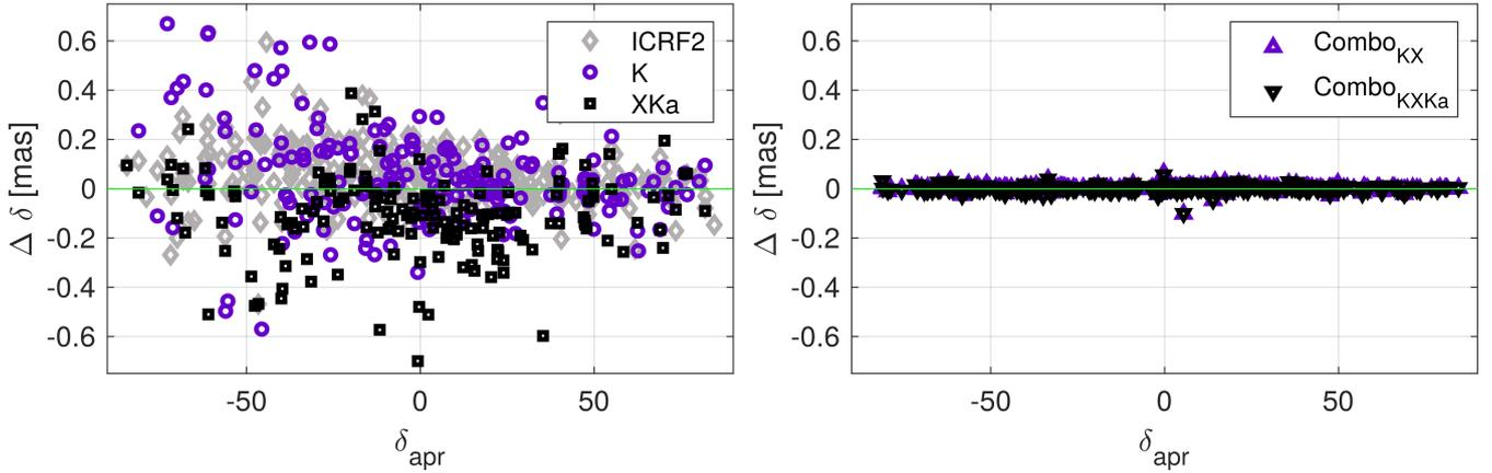
**Fig. 5.** Residuals of the defining sources plotted over declination with respect to ICRF3. *Left:* gray diamonds for ICRF2, purple circles for  $K$  band and black squares for  $XKa$ ; *right:* purple triangles for  $\text{Combo}_{KX}$  and black triangles for  $\text{Combo}_{KXKa}$ .
