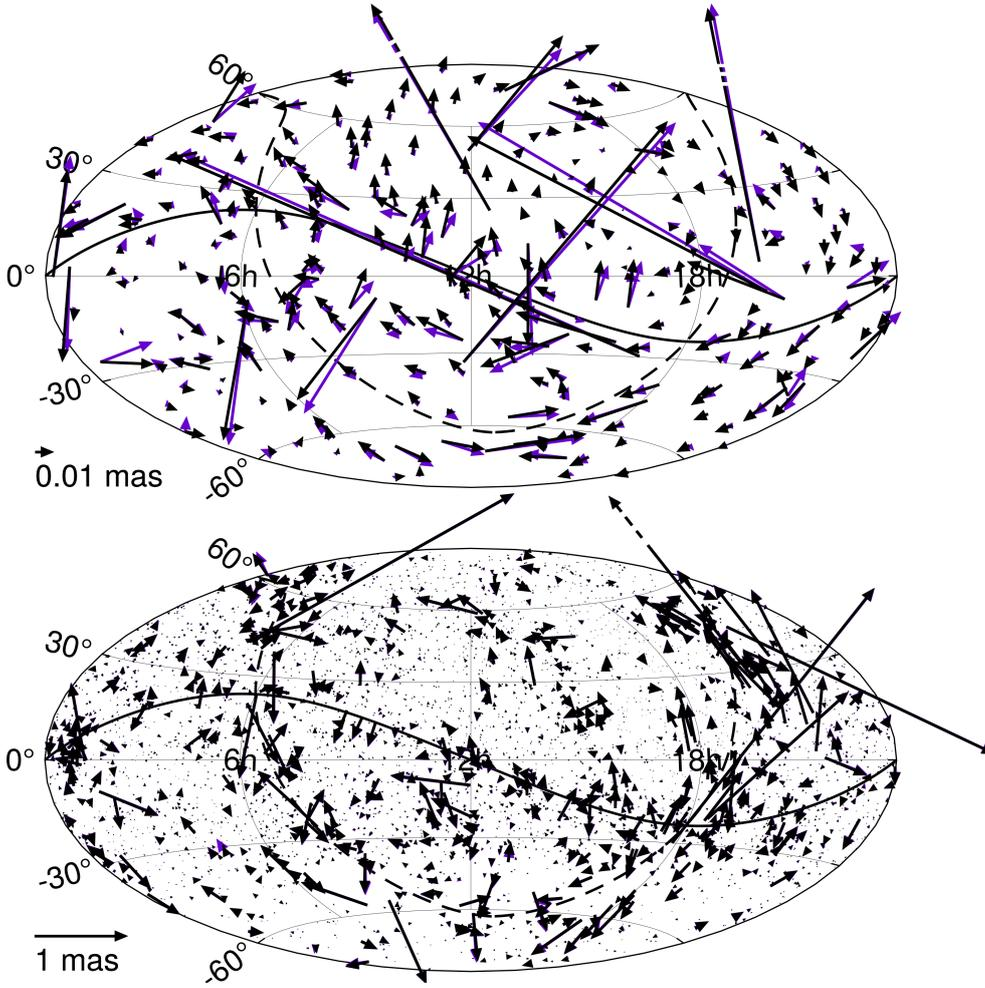
**Fig. 6.** Residuals with respect to ICRF3, shown in purple  $\text{Combo}_{KX}$  and in black  $\text{Combo}_{KXKa}$ . *Top:* ICRF3 defining sources only. *Bottom:* all sources. Sources with residuals  $>2$  mas or  $\sigma > 2$  mas were excluded. The solid line denotes the ecliptic, the dashed line the galactic equator.
