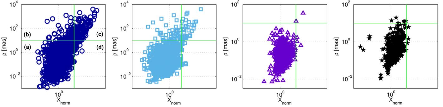
**Fig. 3.** Angular separation  $\rho$  against the normalized separation  $X_{\text{norm}}$  for (from left to right) VIE (dark blue), GFZ (light blue),  $K$  band (purple), and  $XKa$  (black) with respect to GSF. The vertical line is located at  $X_{\text{norm}} = 4.1$ , the horizontal at  $\rho = 10$  mas.
