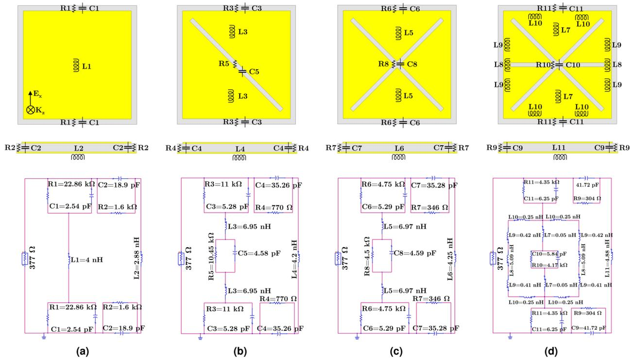
**Figure 5.** Equivalent electrical model for the unit-cell design steps representing the location of the corresponding lumped components in their structures: (a) unslotted patch; (b)–(d) slotted patch with one, two, and three slits, respectively.
