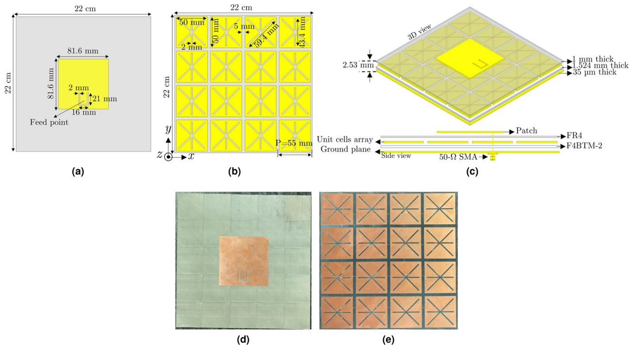
**Figure 1.** Geometry of the proposed metasurface patch antenna: (a) top-view of the patch; (b) top-view of the metasurface structure with 4 × 4 elements; (c) 3D- and side-view of the MPA design; (d) top-view of the fabricated patch; (e) top-view of the metasurface structure prototype.
