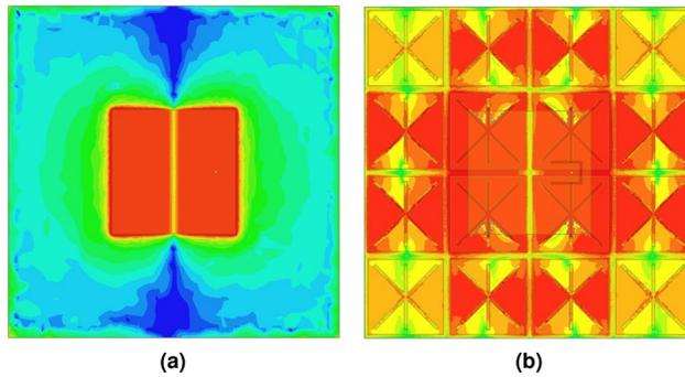
**Figure 10.** E-field distributions under the FR4 layer on the  $x$ - $y$  plane for 1 W input power at 868 MHz for the (a) typical patch antenna; (b) MPA structure. Scale: logarithmic with 15 subdivisions ranging from 1 to  $2 \times 10^3$  V/m.
