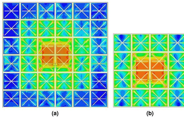
**Figure 7.** Surface current contributions on the unit-cell array at 868 MHz with (a)  $6 \times 6$  and (b)  $4 \times 4$  element matrix. Scale: logarithmic with 15 subdivisions ranging from 0.06 to 60 A/m.
