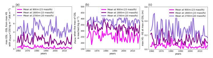
**Figure 10.** Limitation of approximating annual maxima of ground snow load (GSL) from annual maxima of snow depth (HS). (a) Difference between annual maxima of GSL and GSL computed from annual maxima of HS and  $\rho_{\text{SNOW}} = 150 \text{ kg m}^{-3}$ . (b) Snow density when annual maxima of GSL are reached. (c) Difference between annual maxima of HS and HS when annual maxima of GSL are reached.
