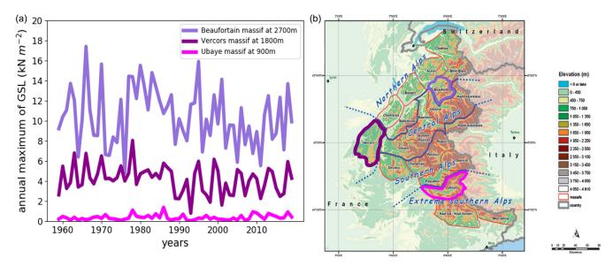
Figure 1. (a) Three time series of annual maxima of ground snow load (GSL) from 1959 to 2019 for 3 massifs at low (900 m), mid (1800 m) or high (2700 m) altitude and (b) 23 mountains massifs of the French Alps and their orographic features (Durand et al., 2009a).
