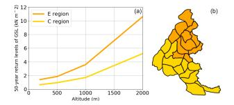
**Figure 2. (a)** French standards 50-year return levels of ground snow load (GSL) with respect to altitude for regions C and E. (b) Map of the region type for each massif.
