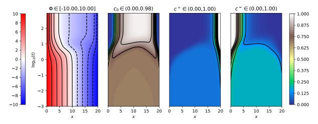
FIGURE 3. Evolution of electrostatic potential  $\Phi$ , solvent concentration  $c_0$ , anion concentration  $c^-$  and cation concentration  $c^+$  for an asymmetric binary electrolyte with equal sizes of solvent molecules, cations and anions.
