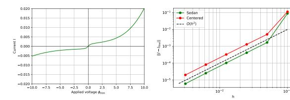
FIGURE 8. Left: Current-voltage curve for electrolytic diode, calculated using the scheme (S). Right: Convergence of calculated IV curve.
