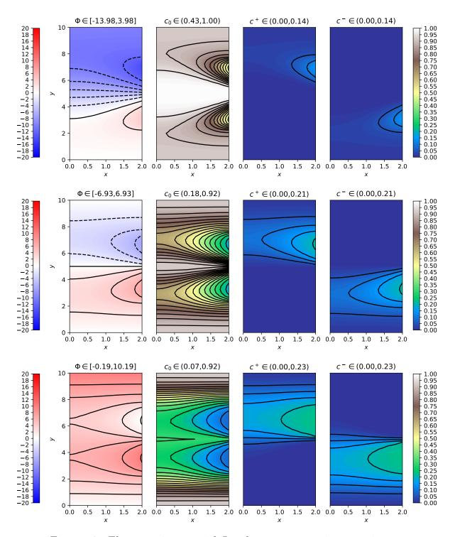
FIGURE 7. Electrostatic potential  $\Phi$ , solvent concentration  $c_0$ , anion concentration  $c^-$  and cation concentration  $c^+$  in an electrolytic diode filled with a symmetric binary electrolyte with equal sizes of solvent molecules at reverse bias  $\Phi_{bias} = -10$  (top), zero bias  $\Phi_{bias} = 0$  (center) and forward bias  $\Phi_{bias} = 10$  (bottom)
