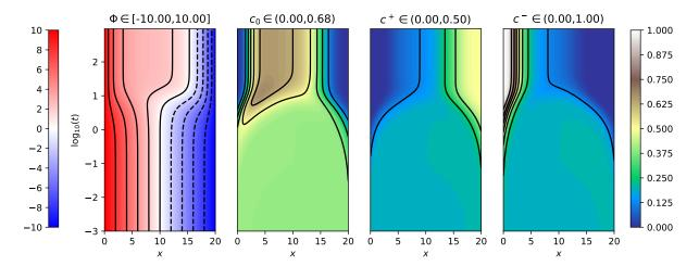
FIGURE 4. Evolution of electrostatic potential  $\Phi$ , solvent concentration  $c_0$ , anion concentration  $c^-$  and cation concentration  $c^+$  for a symmetric binary electrolyte with equal sizes of solvent molecules and anions, but larger cations.
