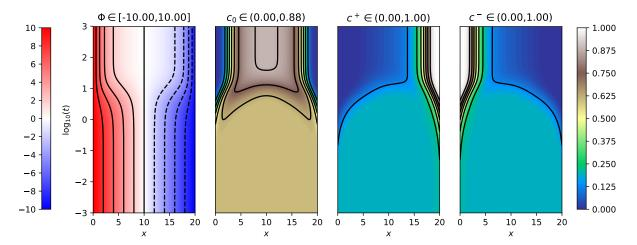
FIGURE 2. Evolution of electrostatic potential  $\Phi$ , solvent concentration  $c_0$ , anion concentration  $c^-$  and cation concentration  $c^+$  for a symmetric binary electrolyte with equal sizes of solvent molecules, anions and cations.
