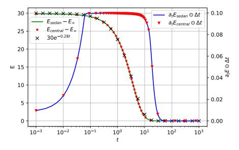
FIGURE 5. Evolution of relative free energy and energy dissipation per time step for symmetric binary electrolyte with equal sizes of solvent molecules and anions, but larger cations.
