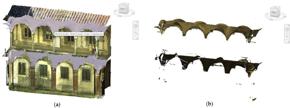
Figure 14. Label 7—Column shaft imported into Recap upfront (a) and later selected on the overall point cloud in Revit (b).
