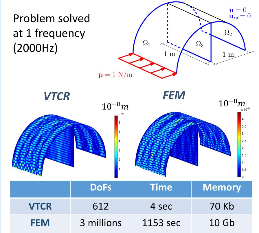
The VTCR is an adapted method for medium frequency
