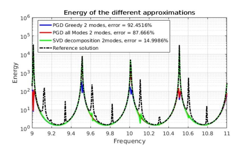
Large band approximated solutions in a square acoustic cavity with different methods (adimensional parameters)
