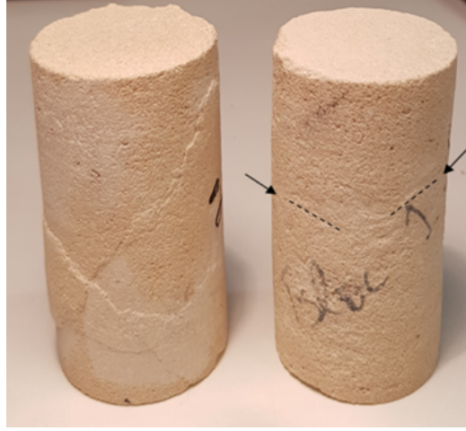
Figure 7: Left: Conjugate shear bands observed at low confining pressure \sigma_3 = -1\text{MPa} ; Right: Deformation bands observed at high confining pressure \sigma_3 = -11\text{MPa} .
