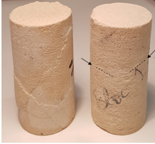
Figure 7: Left: Conjugate shear bands observed at low confining pressure \sigma_3 = -1\text{MPa} ; Right: Deformation bands observed at high confining pressure \sigma_3 = -11\text{MPa} .
