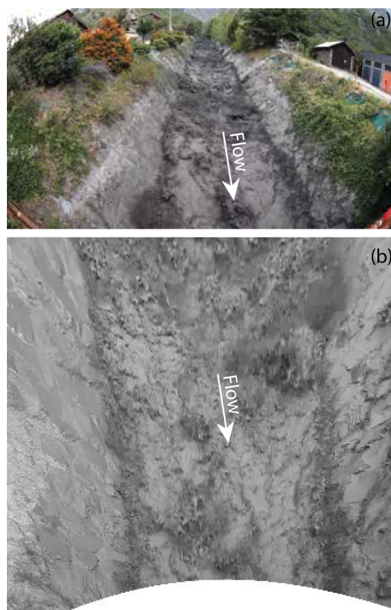
Figure 4. (a) Original footage of a flash flood in the St. Julien torrent acquired by a storm chaser equipped with Canon EOS 5D mark II camera. (b) Orthorectified and geometrically stable image with the field of view clipped to the lower 50 % of the image. The direction of flow is indicated by the arrows.
