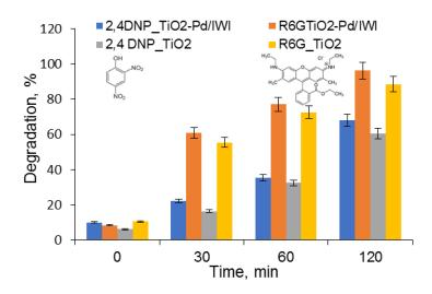
**Figure 10.** 2,4 DNP and rhodamine 6G (R6G) degradation in the presence of  $TiO_2$ -Pd/IWI and  $TiO_2$ . Experimental conditions: photocatalyst dose = 1g/L; pollutant = 20 mg/L.
