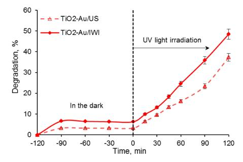
**Figure 6.** 2,4 dinitrophenol (2,4 DNP) degradation (20 mg/L) in the presence of the  $TiO_2$ -Au (1 g/L) catalysts, obtained by US and IWI methods.
