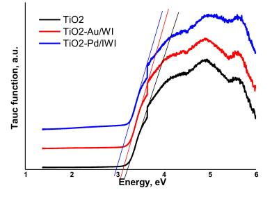
**Figure 5.** Tauc plots for the TiO<sub>2</sub>-derived samples prepared by the IWI method.
