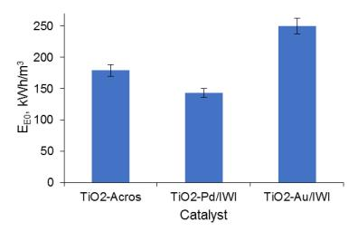
Figure 9. Energy consumption for the obtained catalyst.
