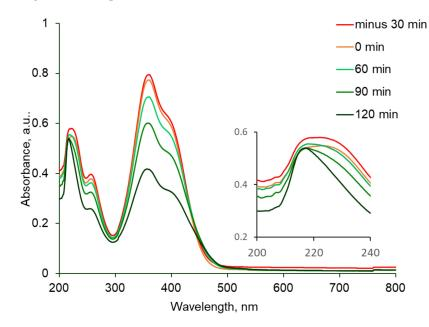
**Figure 7.** Temporal changes in UV-Vis absorption spectra for 2,4 DNP measured at the end of the adsorption reaction and during the photodegradation (20 mg/L) in aqueous solution in the presence of TiO<sub>2</sub>-Au/IWI (1 g/L).
