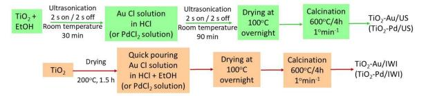
Figure 1. Flow chart of the main steps for the protocols used in this study for catalyst preparation.
