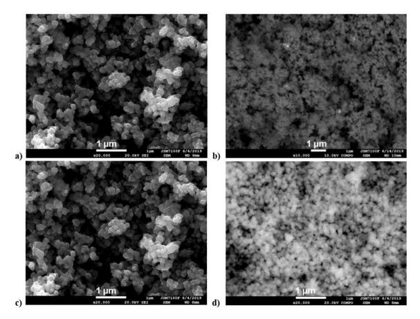
Figure 3. SEM micrographs: (a,b) of TiO<sub>2</sub>-Pd/IWI) and (c,d) TiO<sub>2</sub>-Au/IWI.
