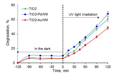
**Figure 8.** 2,4 DNP degradation in aqueous solution in the presence of the  $TiO_2$ -Acros,  $TiO_2$ -Pd and  $TiO_2$ -Au catalysts obtained by the IWI method.
