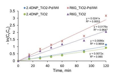
**Figure 11.** Reaction kinetics profiles for the degradation of 2,4 DNP and R6G in the presence of  $TiO_2$ -Pd/IWI and  $TiO_2$ . Experimental conditions: photocatalyst dose = 1g/L; pollutant = 20 mg/L.
