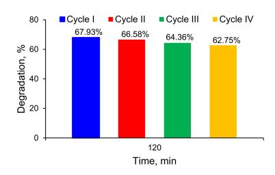
**Figure 12.** Variation of 2,4 DNP photodegradation efficiency within four consecutive reaction cycles on TiO<sub>2</sub>-Pd/IWI.
