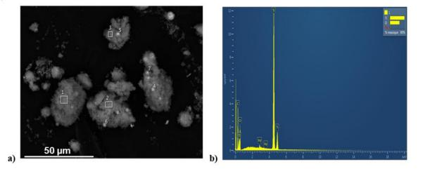
Figure 4. Elemental mapping by EDAX for the  $TiO_2$ -Pd/IWI sample: (a) overall aspect, (b) average elemental composition on the selected areas.
