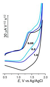
**Figure 7.** Scan rate-normalized voltammograms of oxidation of **9** at a glassy carbon (GC) electrode in AN/0.1 M Bu<sub>4</sub>NPF<sub>6</sub>. Numbers: scan rate v in V s<sup>-1</sup>.
