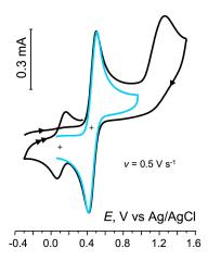
**Figure 9.** Oxidation of ferrocene alone (blue) and in the presence of 7 (black) at a GC electrode in AN/0.1 M Bu<sub>4</sub>NPF<sub>6</sub>. Cross marks show the  $E_0$ s of the two redox systems.
