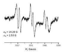
**Figure 10.** EPR spectrum of the spin adduct from the reduction of **7** at a Pt electrode (E = -0.9 V) in the presence of N-*t*-butyl- $\alpha$ -phenylnitrone (PBN). AN/0.1 M Bu<sub>4</sub>NPF<sub>6</sub>.
