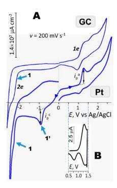
**Figure 8.** Cyclic (**A**) and square-wave (**B**) voltammetry of 7 in AN/0.1 M Bu<sub>4</sub>NPF<sub>6</sub>. T = 20 °C. Anodic and cathodic scans are traced independently.
