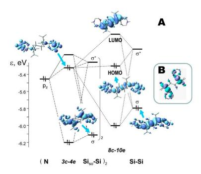
**Figure 11.** (**A**) Two 3c-4e systems of silocane units and resulting nonbonding 8c-10e HOMO in 5 from DFT B3LYP/aug-CC-pVQZ in acetonitrile (C-PCM). (**B**) For comparison, HOMO of 1,4-disilatranyltetrasilane, the Si<sub>4</sub> chain has the same orientation as in (**A**).
