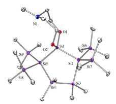
**Figure 4.** Molecular structure of **9** (thermal ellipsoid plot drawn at the 30% probability level). All hydrogen atoms are omitted for clarity (bond lengths in Å, angles in deg). Si(1)-O(1) 1.656(2), Si(1)-O(2) 1.659(2), Si(1)-Si(2) 2.3553(12), Si(3)-C(6) 1.894(3), N(1)-C(4) 1.461(4), O(1)-C(1) 1.426(4), O(2)-C(3) 1.422(3), C(1)-C(2) 1.508(4), O(1)-Si(1)-O(2) 109.92(11), Si(2)-Si(1)-Si(5) 109.59(5), C(21)-N(1)-C(4) 111.6(3), C(4)-N(1)-C(2) 114.8(3).
