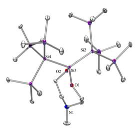
**Figure 2.** Molecular structure of **8** (thermal ellipsoid plot drawn at the 30% probability level). All hydrogen atoms are omitted for clarity (bond lengths in Å, angles in deg). Si(3)-O(1) 1.652(2), Si(3)-O(2) 1.660(2), Si(3)-Si(4) 2.3811(12), Si(3)-Si(2) 2.3881(13), Si(2)-Si(1) 2.3542(14), Si(1)-C(7) 1.887(4), O(1)-C(1) 1.433(4), N(1)-C(4) 1.459(5), C(1)-C(2) 1.510(5), O(1)-Si(3)-O(2) 110.67(12), C(4)-N(1)-C(2) 114.2(3).
