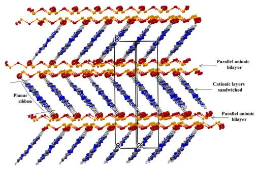
Fig. 3. A view of the crystal packing of (I) showing the stacking of adeninium cations and hydrogen diselenite anions.
