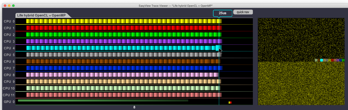
Figure 23: The execution trace of a hybrid OpenCL + OpenMP version of the life kernel allows to make sure that the GPU and the CPU are working in parallel. Data transfers at the end of each iterations also appear in the GPU lane (red = host-to-device transfer, yellow = device-to-host transfer).
