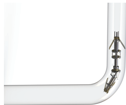
(d) Rear leg declamping, front leg clamping and retracted central module, exit from pipe bend
