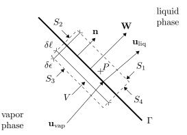
Figure 1: The volume V is a thin band of width  $\delta \epsilon$  and length  $\delta \ell$  centered on the interface  $\Gamma$  moving at velocity  $\mathbf{W} = D\mathbf{n}$ , and delimited by the surface  $S = S_1 \cup \cdots \cup S_4$ . The point P is at rest with respect to the interface.
