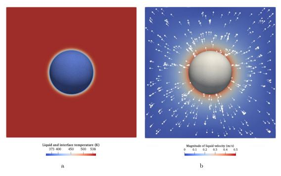
Figure 13: Results in three dimensions on the finest tetrahedral grid used  $(R_1/\Delta x = 53)$ . The threedimensional interface is represented together with a two-dimensional slice of the computational domain. On a, the liquid temperature field is shown at final time. On b, the liquid velocity field is shown at final time. These fields correspond to the simulation illustrated in Fig. 11b.
