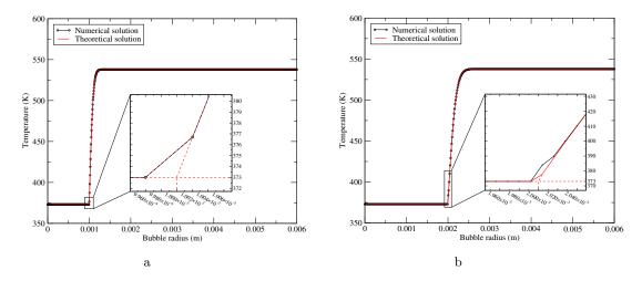
Figure 12: Radial profile of the three-dimensional temperature field shown at a initialization ( $R_0 = 1 \times 10^{-3}$  m) and b final time ( $R_1 = 2 \times 10^{-3}$  m) for  $\Delta x = 3.75 \times 10^{-5}$  m.
