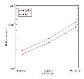
Figure 9: Relative errors on the final bubble radius,  $\xi_2(R)$  and  $\xi_{\infty}(R)$ , for the two-dimensional simulations on unstructured grids illustrated in Fig. 8.
