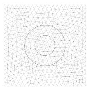
Figure 4: Coarsest grid used in two dimensions ( $\Delta x = 4 \times 10^{-4}$  m) for the simulation of the growth of a static bubble with a constant and uniform mass transfer rate. The small circle represents the initial interface of radius  $R_0 = 1 \times 10^{-3}$  m, whereas the bigger circle represents the final theoretical interface (the radius is twice the initial one).
