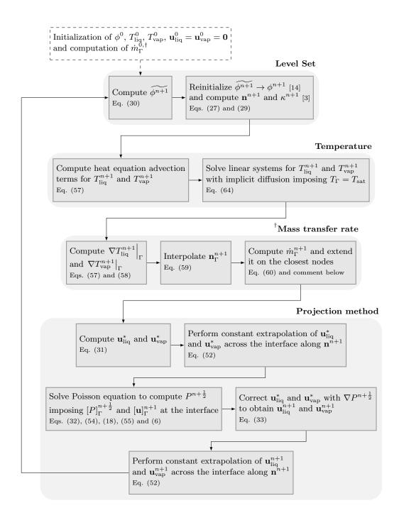
Figure 3: Algorithm used in our solver. The computations of the narrow band around the interface and of the relative distance  $\theta$  are omitted. They are actually performed at initialization, and twice in the temporal loop: once after the advection of the Level Set function and once after its reinitialization. Moreover, the computation of the time step and the exit condition of the temporal loop are also omitted.
