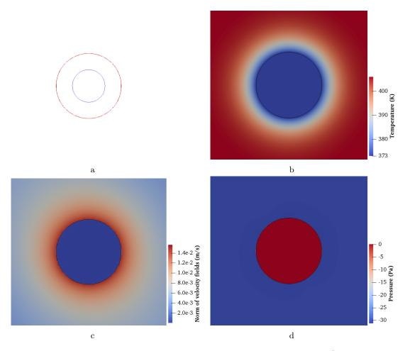
Figure 8: Results in two dimensions on the finest triangular grid used ( $\Delta x = 2.344 \times 10^{-5}$  m). On a, the initial interface is shown in blue, the final computed interface, in black, and the final theoretical interface in red. The final liquid and vapor temperature fields are shown on b, the final velocity fields are shown on c and the final pressure field is shown on d.
