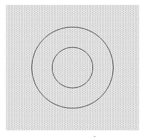
Figure 7: Coarsest two-dimensional grid ( $\Delta x = 9.375 \times 10^{-5} \text{ m}$ ) composed only of equilateral triangles used is our simulations. The small circle represents the initial interface of radius  $R_0 = 1 \times 10^{-3} \text{ m}$ , whereas the bigger circle represents the final theoretical interface (the radius is twice the initial one).
