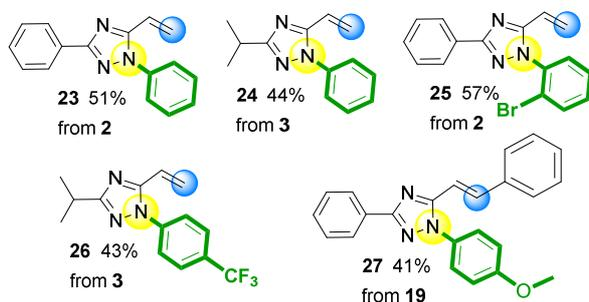
Figure 5. Selective Cu-catalyzed N-arylation of triazoles.
