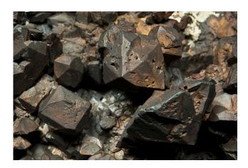
**Figure 2.** Close-up view of the Michigan copper sample (Sorbonne collection no. 9723). The natural  $\{410\}$  tetrahexahedral copper crystals are clearly visible. Field of view:  $7 \times 4.6$  cm. Photo: Alain Jeanne-Michaud.
