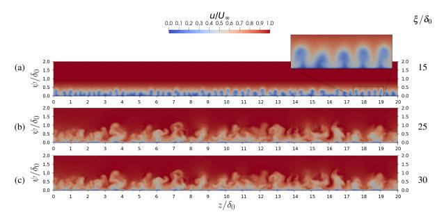
FIG. 6. Instantaneous streamwise velocity field  $u/U_{\infty}$  at  $\xi/\delta_0 = 15$  (a), 25 (b) and 30 (c). In (a) mushroom-like structures of the Görtler instability are evident (see inset for a zoomed view). For  $\xi/\delta_0 > 25$  (b-c), a scale multiplicity is observed in the instantaneous velocity fields (i.e. turbulent state).
