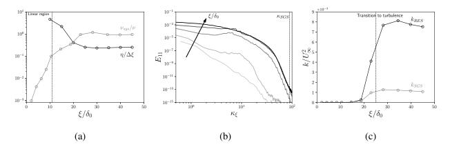
FIG. 2. (a) Ratio between the Kolmogorov scale  $\eta$  and the mesh size in the streamwise direction  $\Delta \xi$  (black line), along with the ratio between the sub-grid viscosity  $v_{SGS}$  and the kinematic viscosity of the fluid v. (b) Streamwise evolution of the energy spectrum  $E_{11}$  for  $\xi/\delta_0=10,15,20,25,35$  (from light grey to black). (c) Streamwise evolution of the explicitly resolved TKE  $k_{RES}$  and the sub-grid TKE  $k_{SGS}$ .
