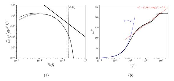
FIG. 3. (a) Normalized energy spectrum for  $\xi/\delta_0 = 35,40,45$  (from light grey to black solid lines), with the -5/3 slope (black solid line) and the Taylor micro-scale (vertical dotted line). (b) Velocity profiles in wall units  $u^+ = f(y^+)$  for  $\xi/\delta_0 = 35,40,45$  (from light grey to black circles).
