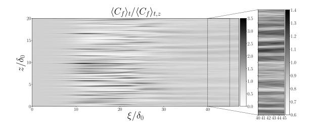
FIG. 11. Curved wall colored by the mean skin friction coefficient  $\langle C_f \rangle_t$  normalized by the local spanwise averaged skin friction coefficient  $\langle C_f \rangle_{t,z}$ . The zoomed area in the inset  $(40 < \xi/\delta_0 < 45)$  highlights the persistence of the heterogeneity in the fully turbulent region.
