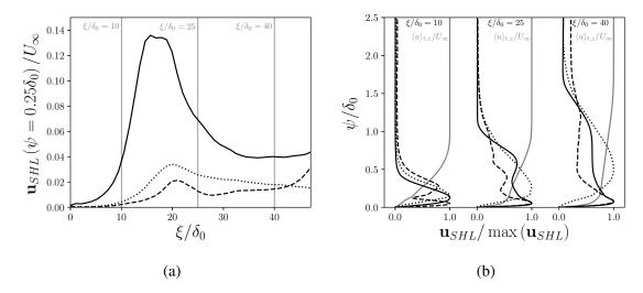
FIG. 7. (a) Streamwise evolution of  $\mathbf{u}_{SHL}$  at  $\psi=0.25\delta_0$  (Eq. 1) for the longitudinal (solid line), wall-normal (dashed line), and spanwise (dotted line) velocity components with the saturation reached at  $\xi/\delta_0\approx 22$ . (b) Selected vertical profiles at  $\xi/\delta_0=(10,25,40)$  (from left to right, respectively) for  $\mathbf{u}_{SHL}$  and normalized by their maximum. The grey solid lines in (b) represent the base state Blasius profile.
