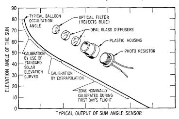
FIGURE 2.—Exploded view of NCAR sun elevation sensor.
