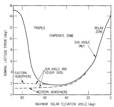
FIGURE 7.—Nominal latitude errors associated with position determination.
