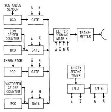
Figure 4.—Logic block diagram of SOMEX II payload (based on NCAR design).
