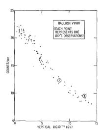
FIGURE 9.—Typical Geiger count rate versus rigidity (calibration curve).
