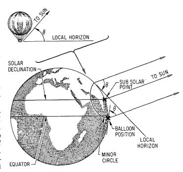
FIGURE 1.—Solar angle method of balloon position determination.
