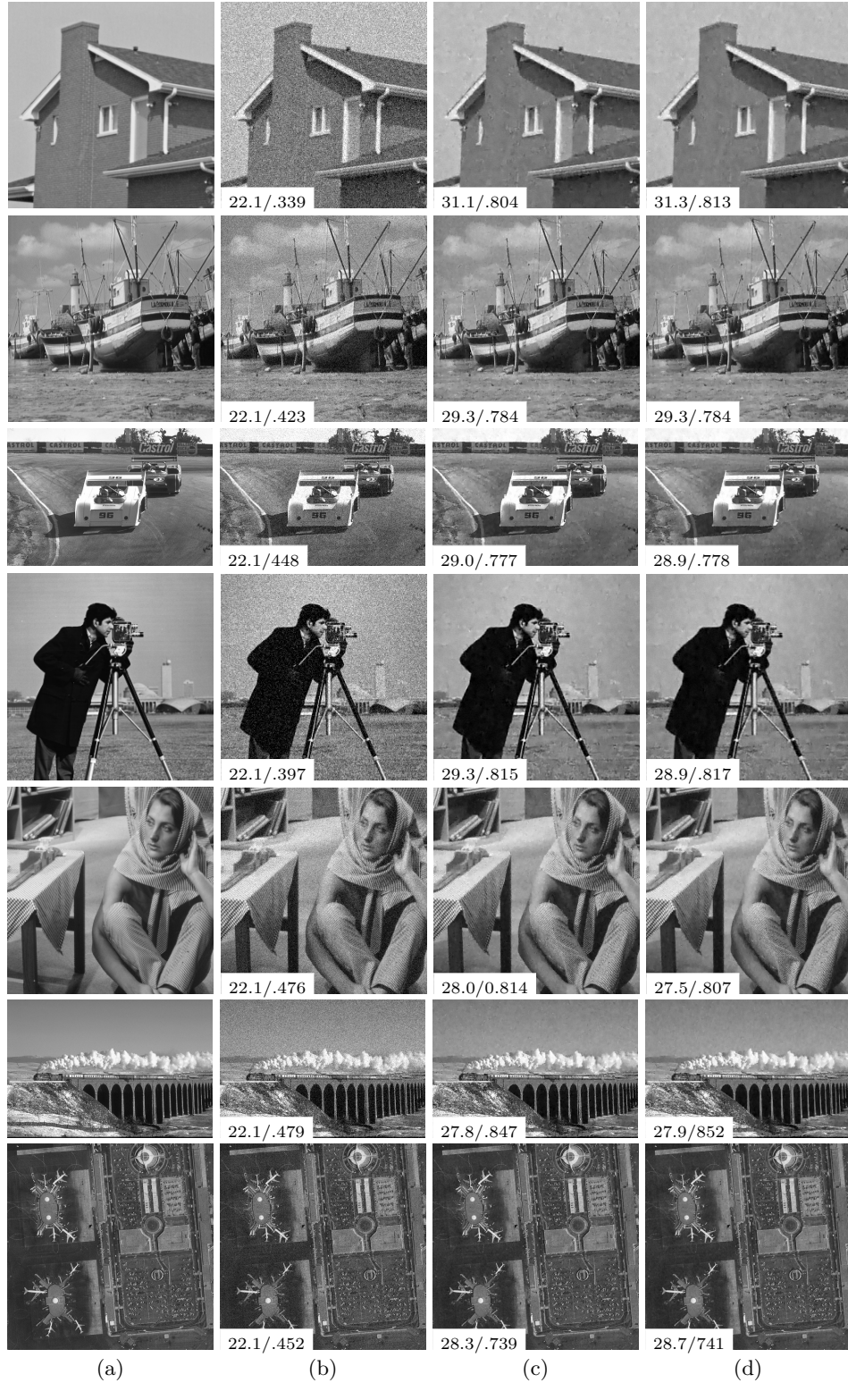
Fig. 3. Denoising results: (a) original, (b) noisy images with \sigma^2 = 20 , (c) results with truncated EM model, (d) results LR-COMP model with PSNR/SSIM. Similar denoising performances are obtained with LR-COMP with a compressed database 250 times smaller.
